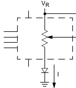
Two terminal Variable Resistor;
