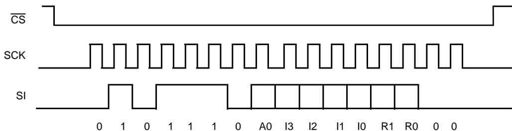
Figure 5. Three-Byte Instruction Sequence (Write)
