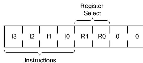
The four high order bits of the instruction byte specify the operation. The next two bits ( $R_1$  and  $R_0$ ) select one of the four registers that is to be acted upon when a register oriented instruction is issued. The last two bits are defined as 0.
