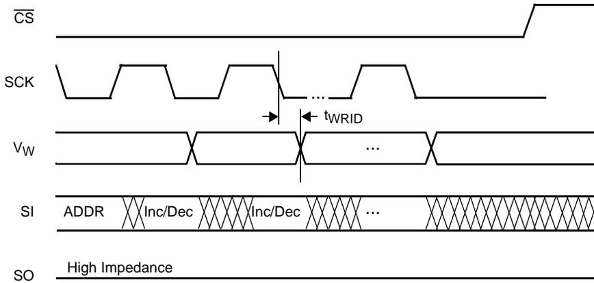
**Write Protect and Device Address Pins Timing**
