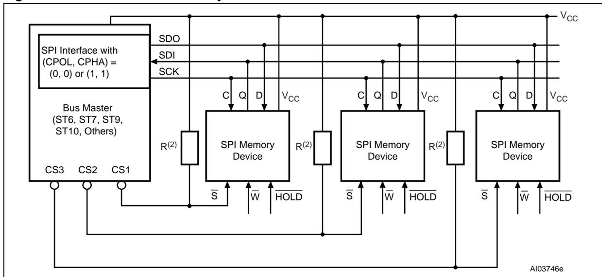
1. The Write Protect ( $\bar{W}$ ) and Hold ( $\bar{HOLD}$ ) signals should be driven, High or Low as appropriate.
