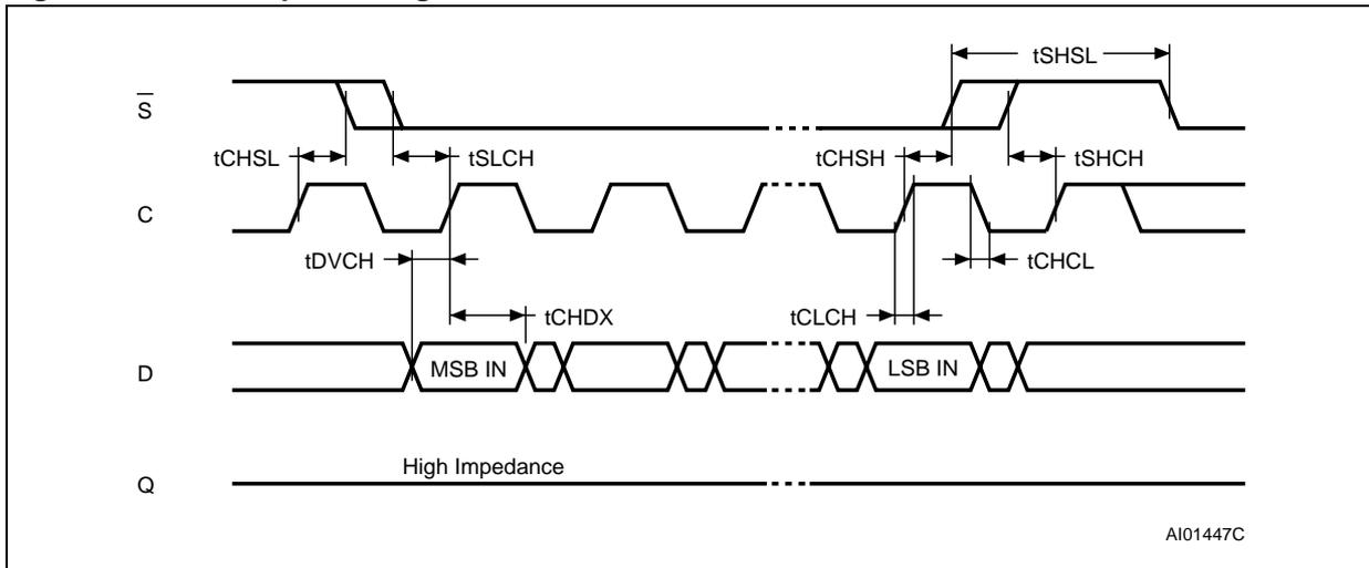
Figure 21. Write Protect Setup and Hold Timing during WRSR when SRWD=1
