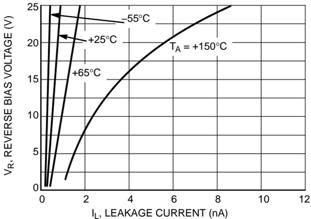
Figure 5.  $I_R$  versus Temperature Characteristics of the NUP2105L
