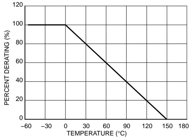
Figure 6. Temperature Power Dissipation Derating of the NUP2501L
