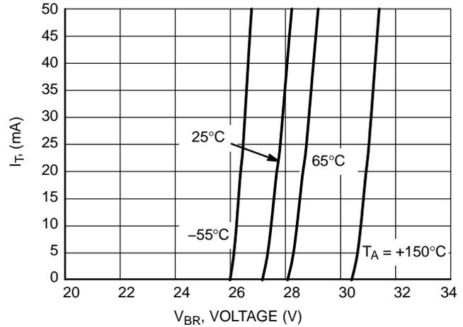
Figure 4.  $V_{BR}$  versus  $I_T$  Characteristics of the NUP2105L
