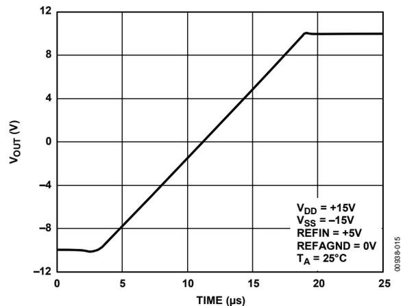
Figure 15. Settling Time
