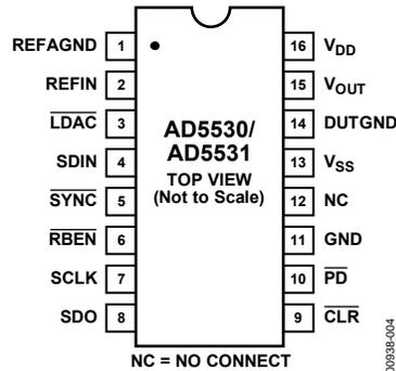
Figure 4. Pin Configuration
