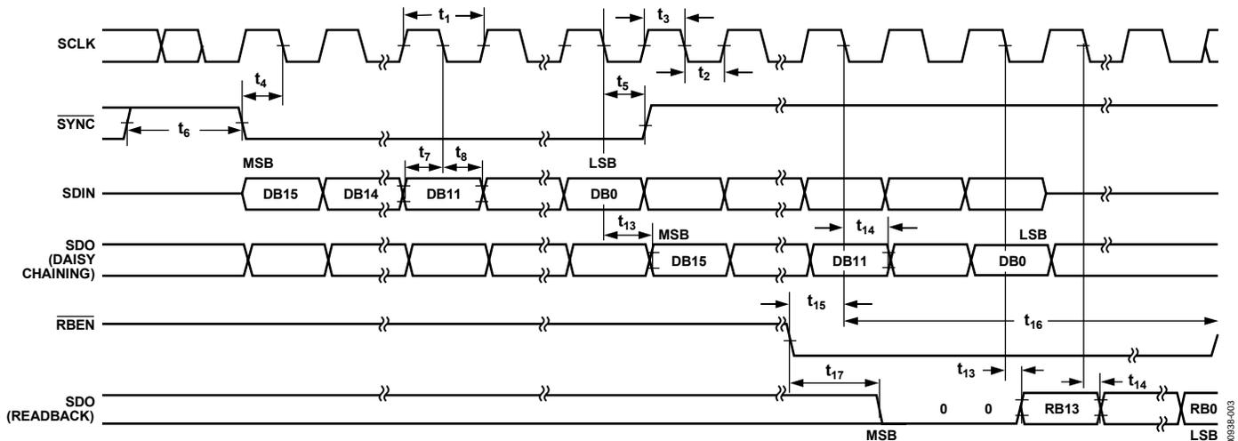
Figure 3. Timing Diagram for Daisy-Chaining and Readback Mode
