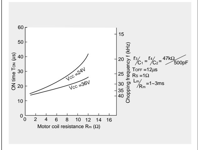
**Chopper frequency vs. Supply voltage**
