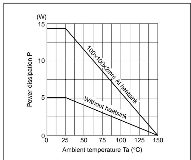
When selecting a heatsink for SLA5017, be sure to check the product temperature when in use in an actual application.
