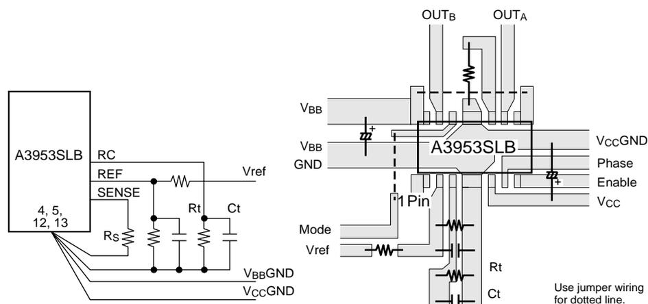
In stepper-motor applications applying a constant current to the load, slow-decay mode PWM is typically used to limit the switching loss in the device and iron losses in the motor.
