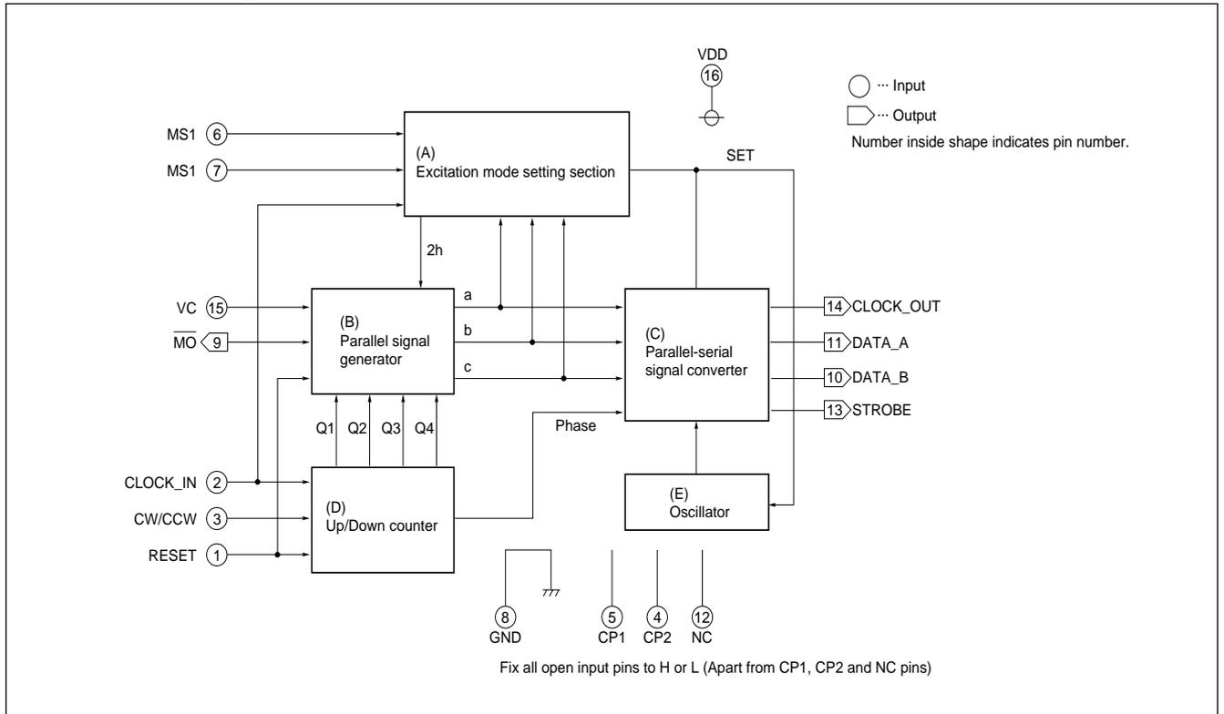
Diagram of Standard External Circuit
