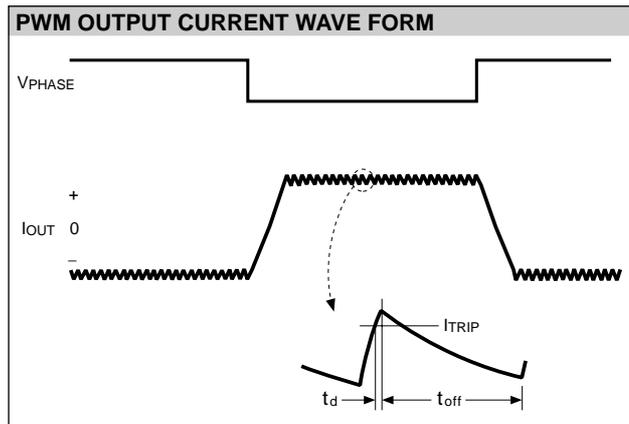
When the bridge is turned ON, current increases in the motor winding and it is sensed by the external sense resistor until the sense voltage ( $V_{SENSE}$ ) reaches the level set at the comparator's input:
