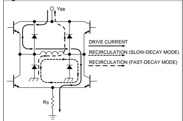
The user selects an external resistor ( $R_T$ ) and capacitor ( $C_T$ ) to determine the time period ( $t_{OFF}=R_T \cdot C_T$ ) during which the drivers remain disabled (see "RC Fixed Off-time" below). At the end of the RC interval, the drivers are enabled allowing the load current to increase again. The PWM cycle repeats, maintaining the peak load current at the desired value (see figure 2).
