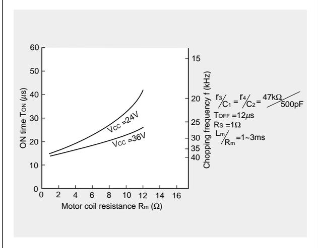
**Chopper frequency vs. Supply voltage**
