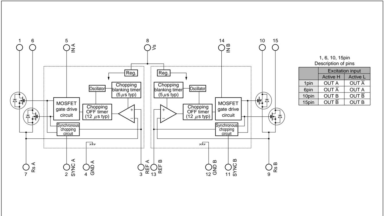
Diagram of Standard External Circuit (Recommended Circuit Constants)
