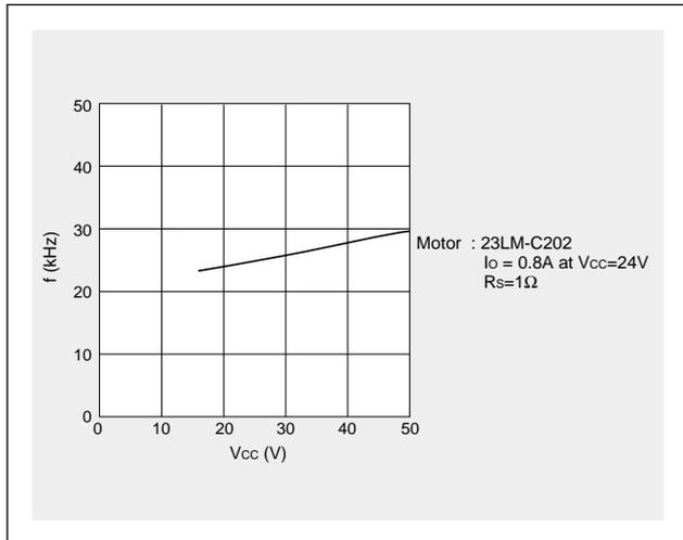
■Chopper frequency vs. Output current
