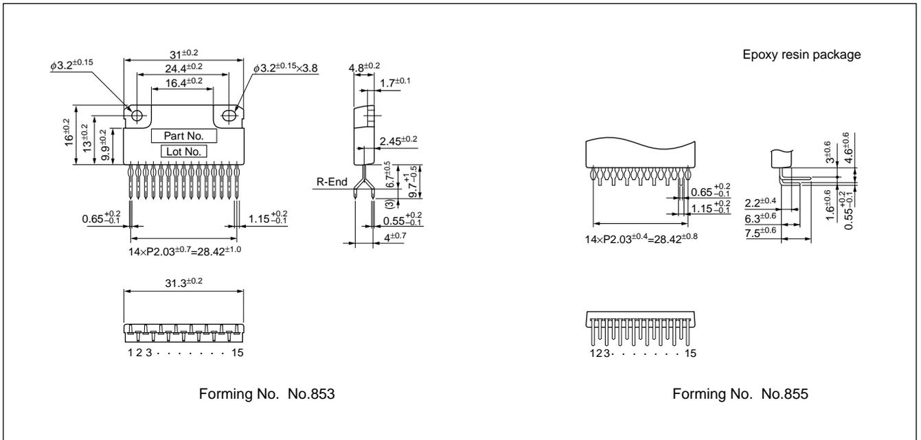
External Dimensions SMA7022MU/SMA7029MA
