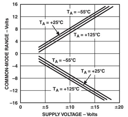
TPC 27. Common-Mode Input Range vs. Supply Voltage
