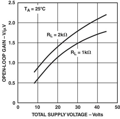
TPC 19. Open-Loop Voltage Gain vs. Supply Voltage
