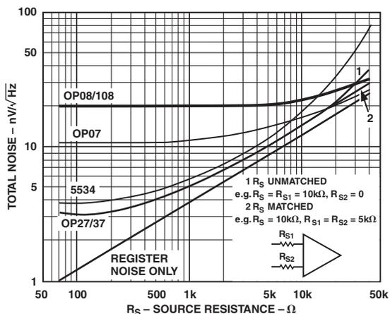
Figure 5. Noise vs. Resistance (Including Resistor Noise @ 1000 Hz)
