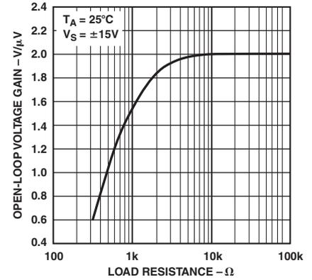
TPC 30. Open-Loop Voltage Gain vs. Load Resistance
