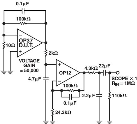
TPC 28. Noise Test Circuit (0.1 Hz to 10 Hz)
