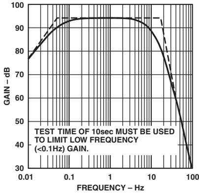
TPC 1. Noise-Tester Frequency Response (0.1 Hz to 10 Hz)
