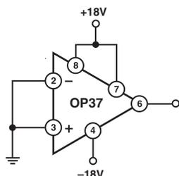
Figure 3. Burn-In Circuit
