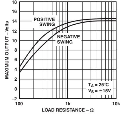
TPC 21. Maximum Output Voltage vs. Load Resistance
