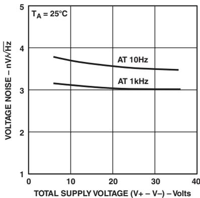
TPC 7. Voltage Noise Density vs. Supply Voltage
