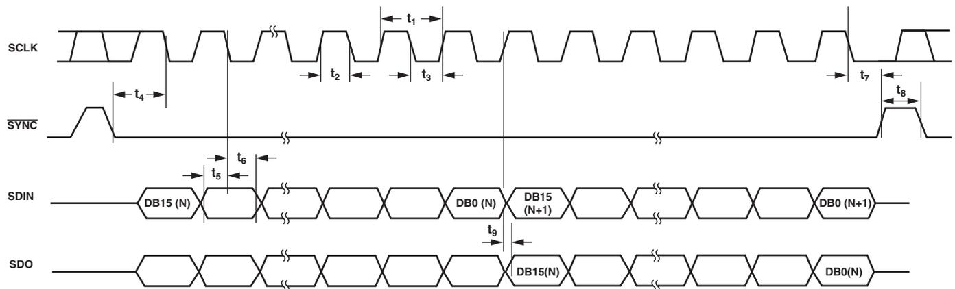
ALTERNATIVELY, DATA MAY BE CLOCKED INTO INPUT SHIFT REGISTER ON RISING EDGE OF SCLK AS DETERMINED BY CONTROL BITS. IN THIS CASE, DATA WOULD BE CLOCKED OUT OF SDO ON FALLING EDGE OF SCLK. TIMING AS PER ABOVE, WITH SCLK INVERTED.
