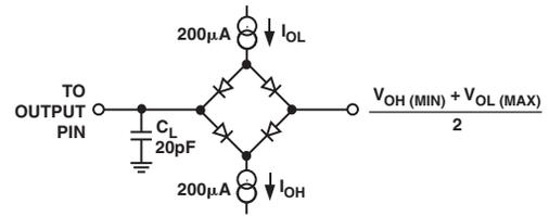
Figure 3. Load Circuit for SDO Timing Specifications
