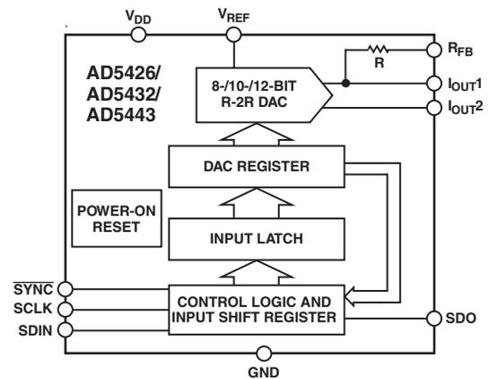
The applied external reference input voltage ( $V_{\text{REF}}$ ) determines the full-scale output current. An integrated feedback resistor ( $R_{\text{FB}}$ ) provides temperature tracking and full-scale voltage output when combined with an external current to voltage precision amplifier.
