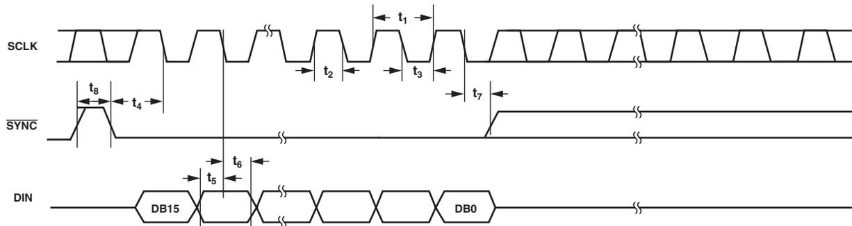
ALTERNATIVELY, DATA MAY BE CLOCKED INTO INPUT SHIFT REGISTER ON RISING EDGE OF SCLK AS DETERMINED BY CONTROL BITS. TIMING AS PER ABOVE, WITH SCLK INVERTED.
