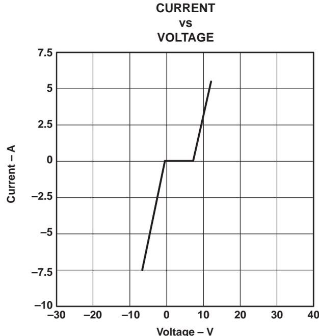
NOTE A: Typical current versus voltage curve was derived using the IEC 1.2/50- $\mu$ s surge waveform.
