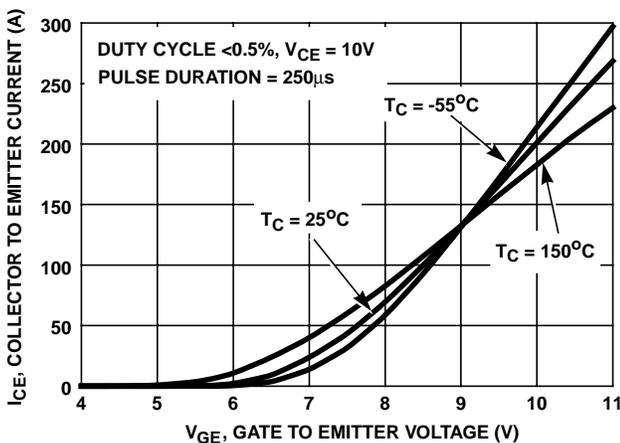
FIGURE 13. TRANSFER CHARACTERISTIC
