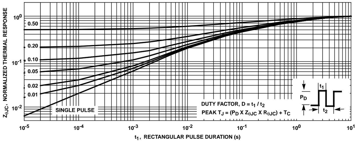
FIGURE 16. NORMALIZED TRANSIENT THERMAL RESPONSE, JUNCTION TO CASE
