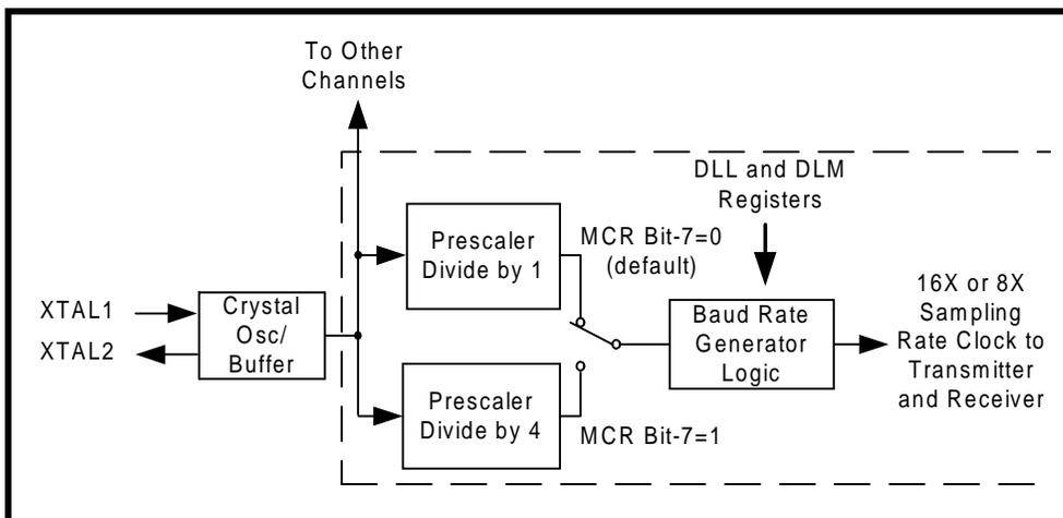
Programming the Baud Rate Generator Registers DLM and DLL provides the capability of selecting the operating data rate. Table 4 shows the standard data rates available with a 14.7456 MHz crystal or external clock at 16X clock rate. At 8X sampling rate, these data rates would double. When using a non-standard data rate crystal or external clock, the divisor value can be calculated for channel 'N' with the following equation(s).
