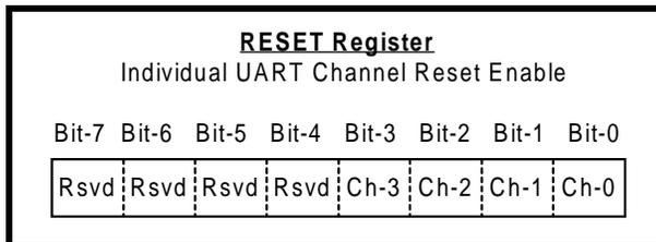
The 8-bit Reset register [RESET] provides the software with the ability to reset individual UART(s) when there is a need. Each bit is self-resetting after it is written a logic 1 to perform a reset to that channel. All registers in that channel will be reset to the default condition, see Table 19 for details. As an example, bit-0 =1 resets UART channel 0 with bit-3=1 resets channel 3.
