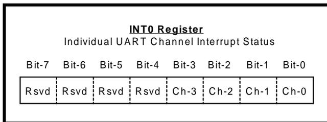
For example, bit-0 represents channel 0 and bit-3 indicates channel 3. Bits 4 to 7 are reserved and remains at logic zero. Logic one indicates the channel N [3:0] has called for service. The interrupt bit clears after reading the appropriate register of the interrupting UART channel register (ISR, LSR and MSR). See Table 13 for interrupt clearing details.
