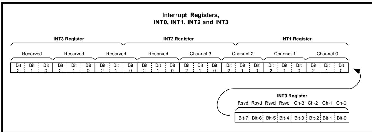
**TABLE 9: UART CHANNEL [3:0] INTERRUPT SOURCE ENCODING AND CLEARING**
