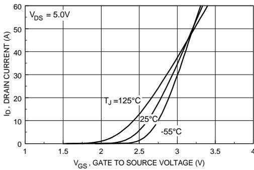
Figure 5. Transfer Characteristics.
