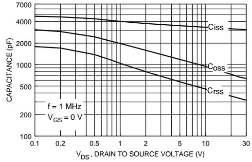
Figure 8. Capacitance Characteristics.
