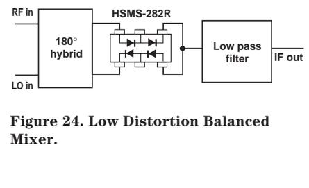
Figure 24. Low Distortion Balanced Mixer.
