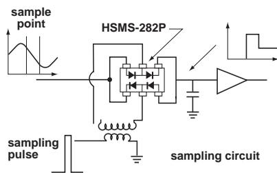
Figure 25. Sampling Circuit.
