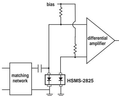
Figure 13. Differential Detector.
