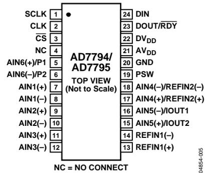
Figure 5. Pin Configuration
