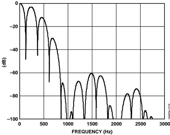
Figure 15. Filter Profile with Update Rate = 242 Hz (Chop Enabled)
