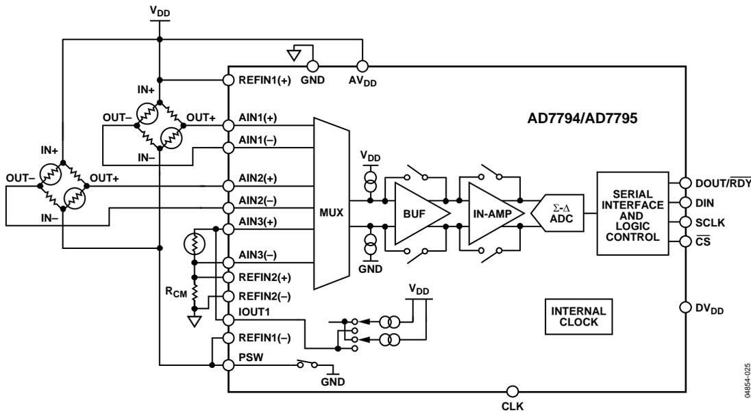
Figure 24. Typical Application (Flowmeter)
