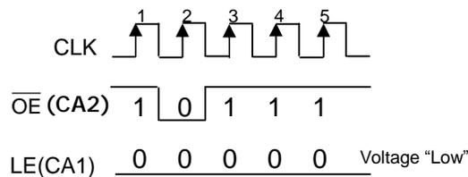
Each time the system controller sends the sequence patterns shown above, MBI5170 can resume to a Normal mode. During this phase, the system controller can still send data through SDI pin.
