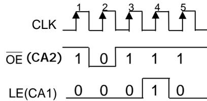
The signal sequence makes MBI5170 enter a **Current Adjust** mode.
