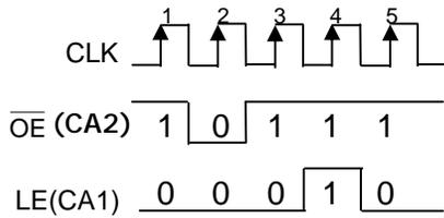
Each time the system controller sends the sequence patterns shown above, MBI5170 can enter the Current Adjust mode. During this phase, the system controller can still send data through SDI pin.
