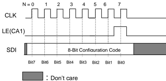
After entering the Current Adjust mode, the system controller sends a 7-bit Current Adjust code to 8-bit Shift Register through MBI5170 SDI pin. Then sending LE(CA1) will transfer the contents in the Shift Register to a 8-bit Configuration Latch rather than the 8-bit Output Latch in a Normal mode. The 7-bit Current Adjust code in the Configuration Latch will directly affect the  $I_O$  Regulator by a gain, G. The output current resulted by the gain values will be then defined as:
