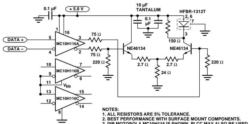
**Figure 5. Recommended Transmitter Drive and Test Circuit.**
