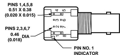
HFBR-2316T is pin compatible with HFBR-24X6 receivers and can be used to extend the distance of an existing application by substituting the HFBR-2316T for the HFBR-2416.
