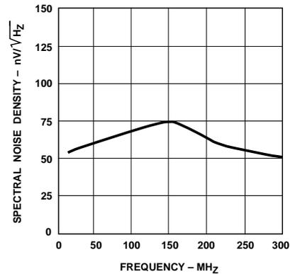
Figure 7. Typical Output Spectral Noise Density vs. Frequency.
