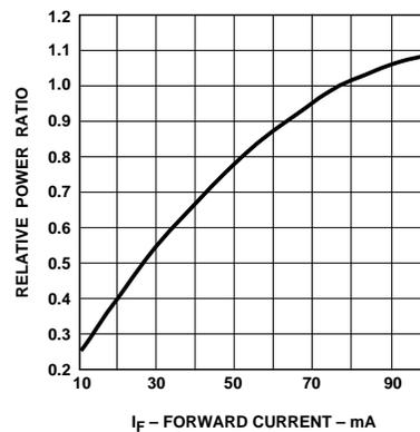
**Figure 4. Normalized Transmitter Output Power vs. Forward Current.**
