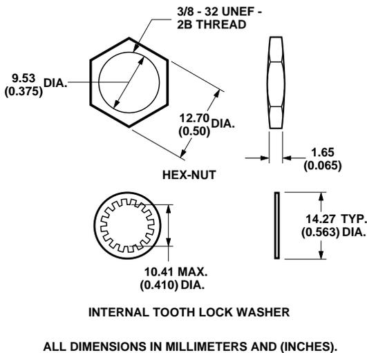
Figure 1. HFBR-4411 Mechanical Dimensions.
