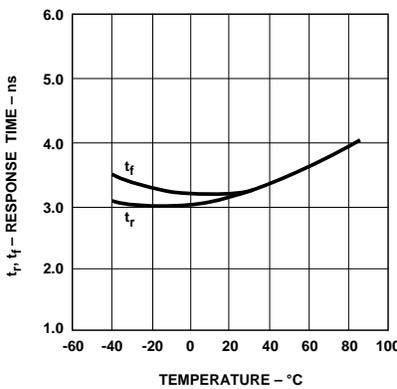
Figure 9. Typical Rise and Fall Times vs. Temperature.
