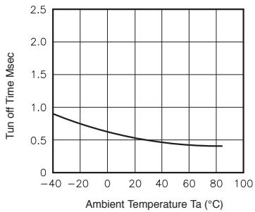
**Fig.5** LED operate vs. ambient temperature
