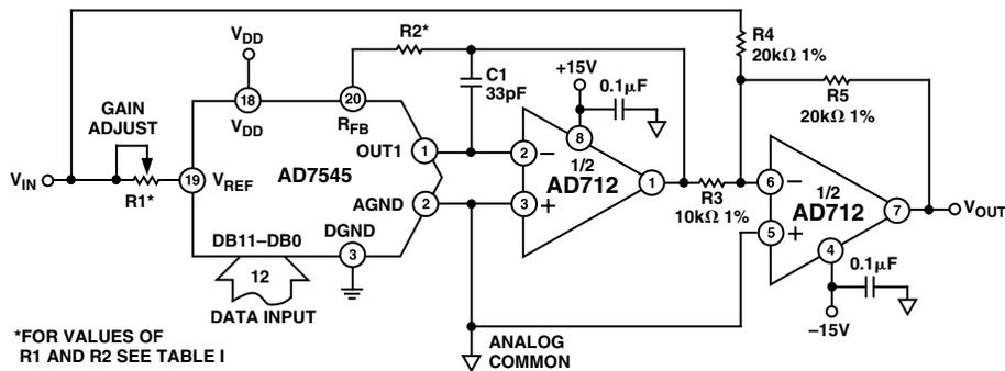
Figure 9. Bipolar Operation
