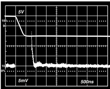
Figure 5b. Settling Characteristics 0 V to -10 V Step
