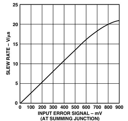
TPC 18. Slew Rate vs. Input Error Signal
