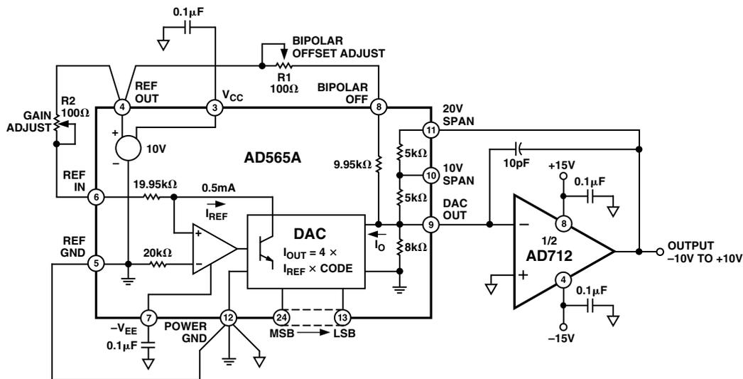
Figure 1. ±10 V Voltage Output Bipolar DAC
