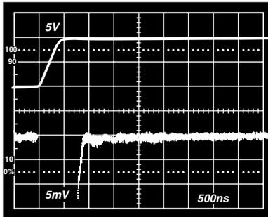
Figure 5a. Settling Characteristics 0 V to +10 V Step
