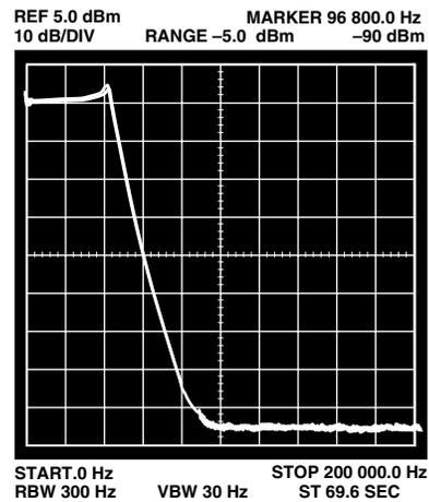
Figure 19. High Frequency Response for 9-Pole Chebyshev Filter
