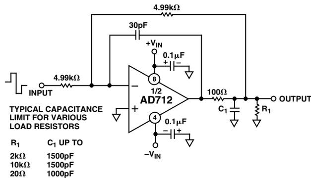
Figure 13. Circuit for Driving a Large Capacitive Load
