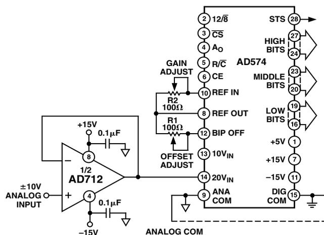
Figure 11. AD712 as ADC Unity Gain Buffer
