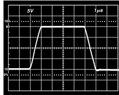
Figure 14. Transient Response R<sub>L</sub> = 2 kΩ, C<sub>L</sub> = 500 pF
