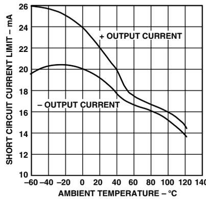
TPC 8. Short Circuit Current Limit vs. Temperature
