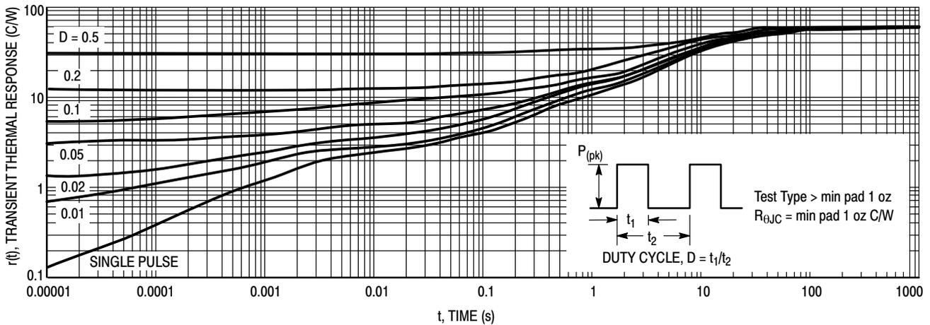
Figure 10. Thermal Response – MBR540PT3G, NRVS540T3G on 1" pad
