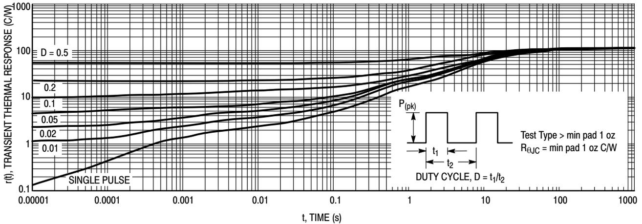
Figure 9. Thermal Response – MBR540PT3G, NRVS540T3G on min pad
