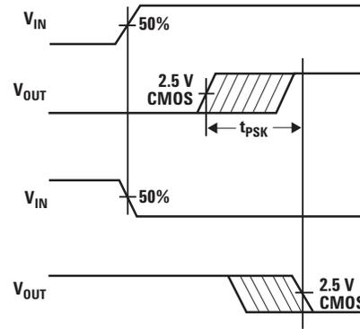
Figure 4. Timing Diagrams to Illustrate Propagation Delay Skew.
