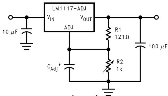
$$V_{OUT} = 1.25 \left( 1 + \frac{R_2}{R_1} \right)$$
