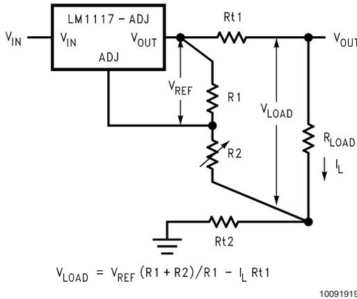
**FIGURE 3. Best Load Regulation using Adjustable Output Regulator**
