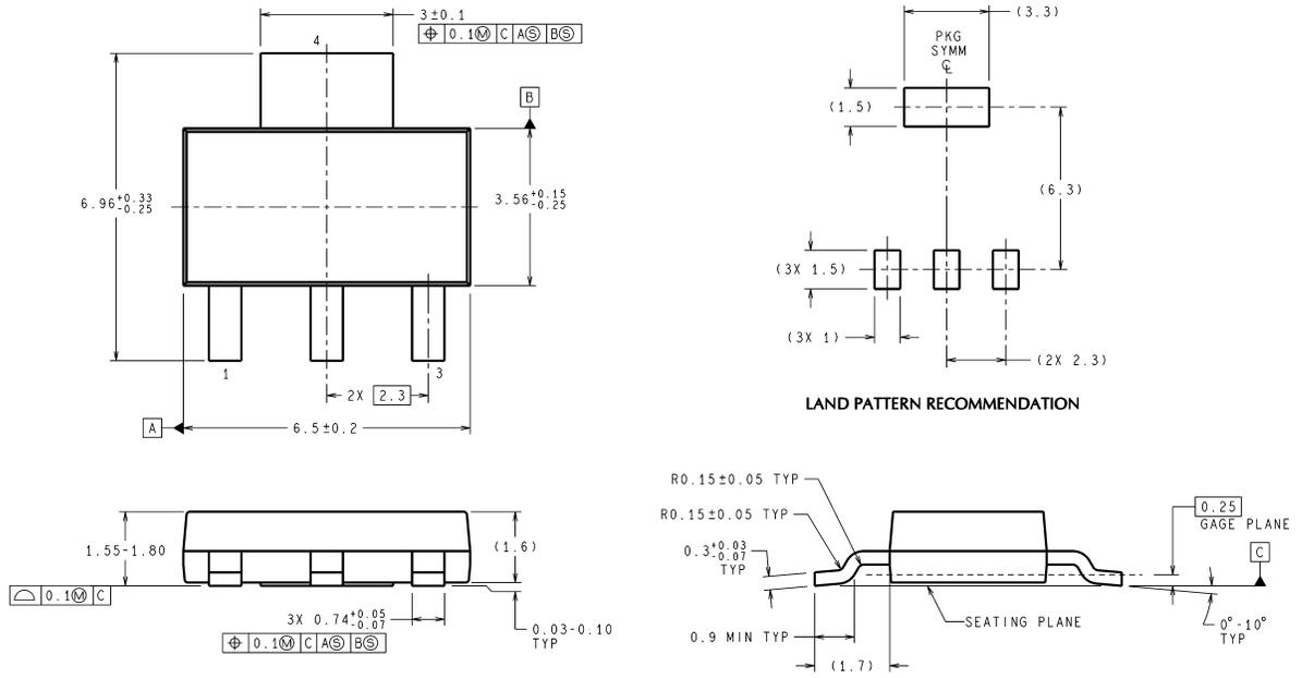
DIMENSIONS ARE IN MILLIMETERS
