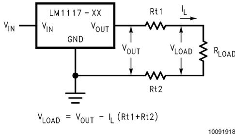
**FIGURE 2. Typical Application using Fixed Output Regulator**
