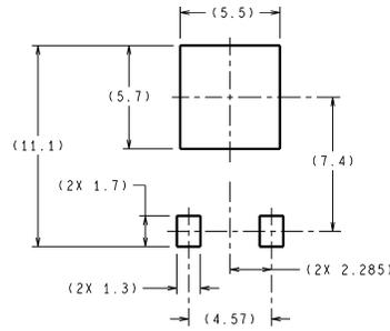
DIMENSIONS ARE IN MILLIMETERS
