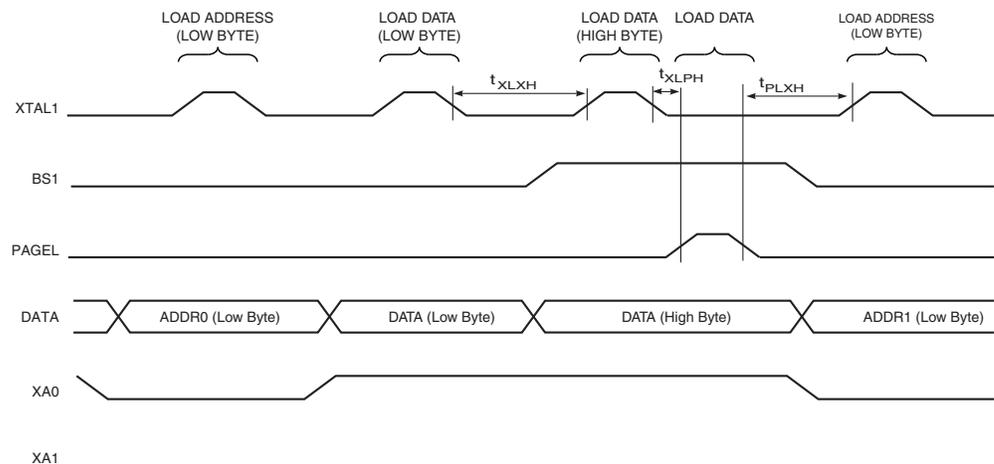
Note: 1. The timing requirements shown in Figure 133 (that is,  $t_{DVXH}$ ,  $t_{XHXL}$ , and  $t_{XLDX}$ ) also apply to loading operation.
