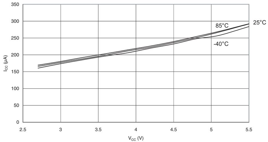
**Figure 208.** Aref External Reference Current vs.  $V_{CC}$
