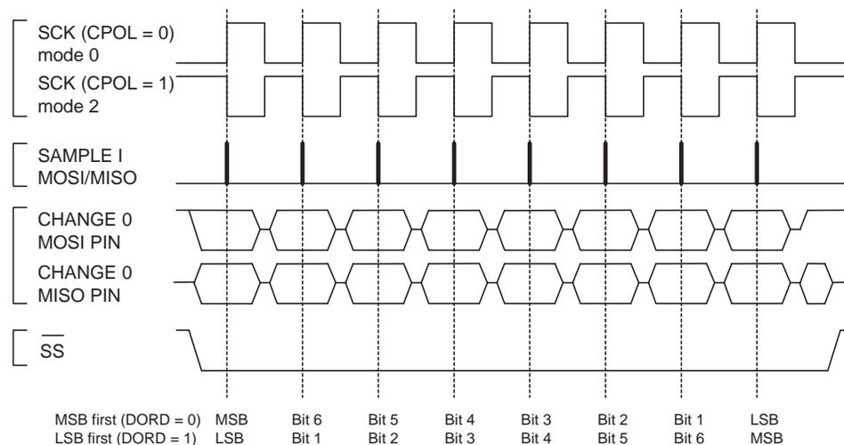
**Figure 68.** SPI Transfer Format with CPHA = 1
