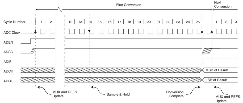
**Figure 102.** ADC Timing Diagram, Single Conversion
