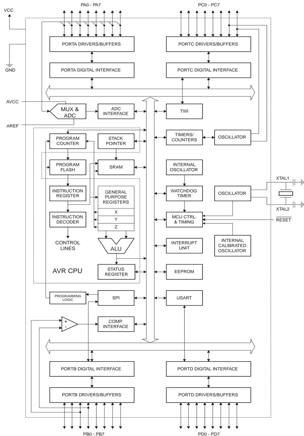
The AVR core combines a rich instruction set with 32 general purpose working registers. All the 32 registers are directly connected to the Arithmetic Logic Unit (ALU), allowing two independent registers to be accessed in one single instruction executed in one clock cycle. The resulting architecture is more code efficient while achieving throughputs up to ten times faster than conventional CISC microcontrollers.
