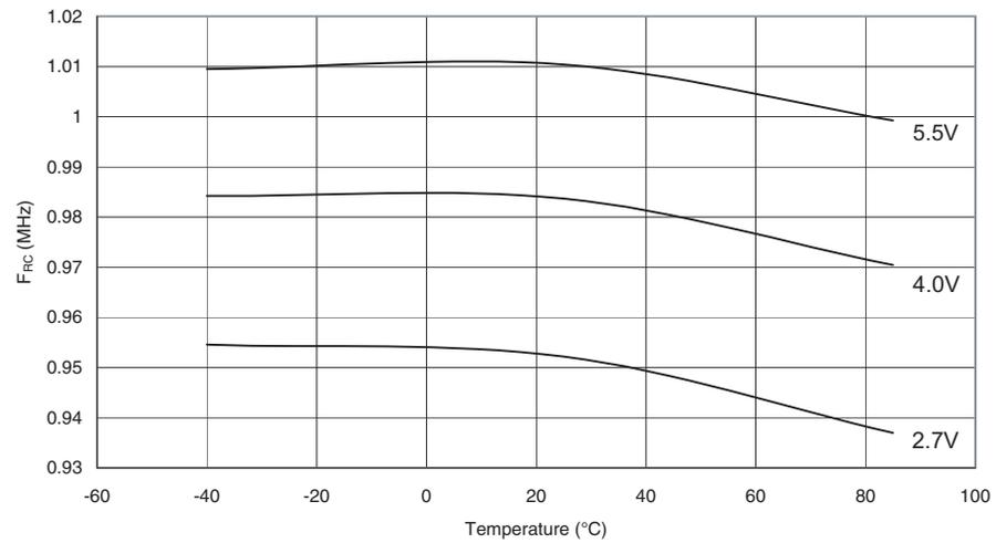
**Figure 204.** Calibrated 1 MHz RC Oscillator Frequency vs.  $V_{CC}$
