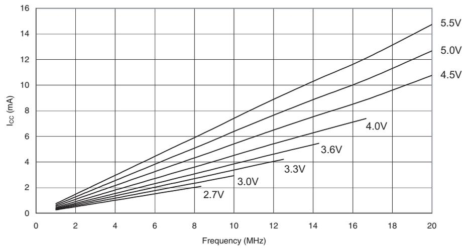
**Figure 158.** Idle Supply Current vs.  $V_{CC}$  (Internal RC Oscillator, 8 MHz)
