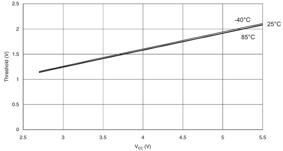
**Figure 183.** I/O Pin Input Threshold Voltage vs.  $V_{CC}$  ( $V_{IL}$ , I/O Pin Read As '0')
