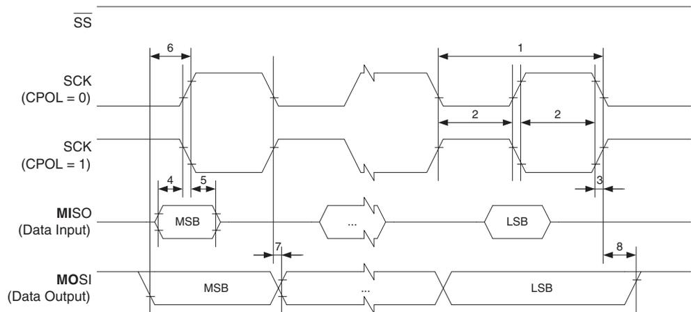
**Figure 148. SPI Interface Timing Requirements (Slave Mode)**
