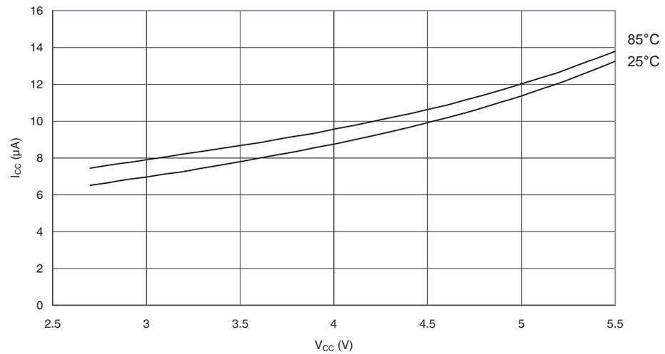
**Figure 210.** Watchdog Timer Current vs.  $V_{CC}$
