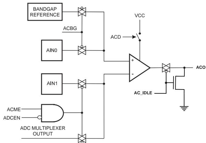
**Figure 122.** General Boundary-scan Cell used for Signals for Comparator and ADC
