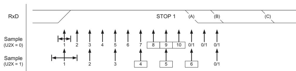
The same majority voting is done to the stop bit as done for the other bits in the frame. If the stop bit is registered to have a logic 0 value, the Frame Error (FE) Flag will be set.
