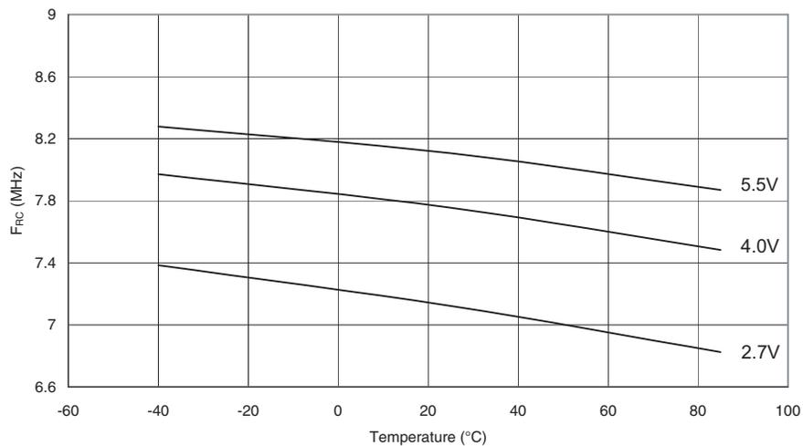
**Figure 195.** Calibrated 8 MHz RC Oscillator Frequency vs. V<sub>CC</sub>
