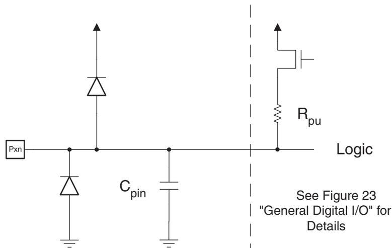
All registers and bit references in this section are written in general form. A lower case “x” represents the numbering letter for the port, and a lower case “n” represents the bit number. However, when using the register or bit defines in a program, the precise form must be used, that is, PORTB3 for bit no. 3 in Port B, here documented generally as PORTxn. The physical I/O Registers and bit locations are listed in “Register Description for I/O Ports” on page 66.
