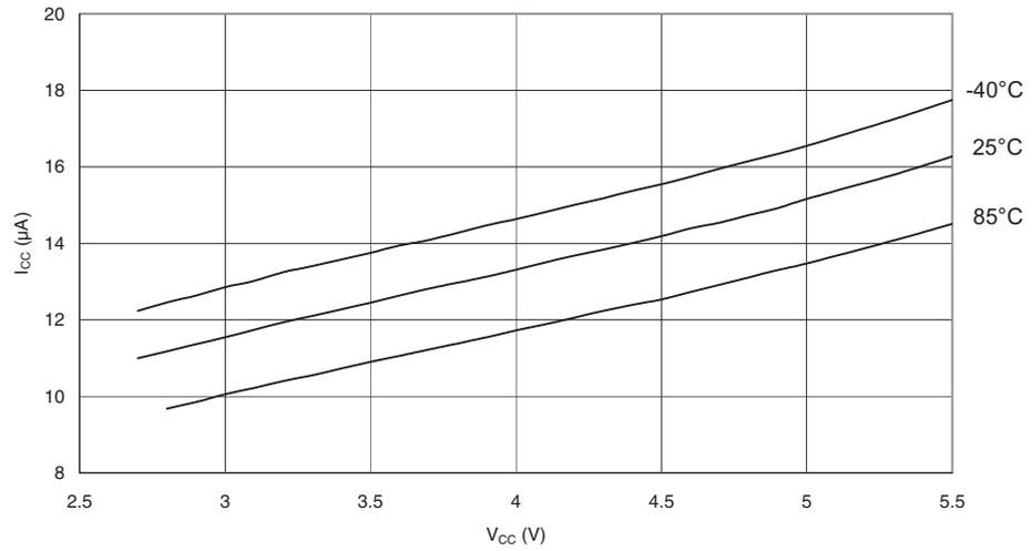
**Figure 207.** ADC Current vs.  $V_{CC}$  (Aref = AVCC)
