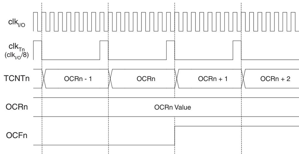
Figure 37 shows the setting of OCF0 and the clearing of TCNT0 in CTC mode.
