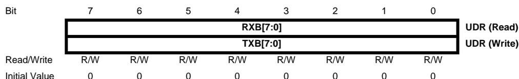
The USART Transmit Data Buffer Register and USART Receive Data Buffer Registers share the same I/O address referred to as USART Data Register or UDR. The Transmit Data Buffer Register (TXB) will be the destination for data written to the UDR Register location. Reading the UDR Register location will return the contents of the Receive Data Buffer Register (RXB).
