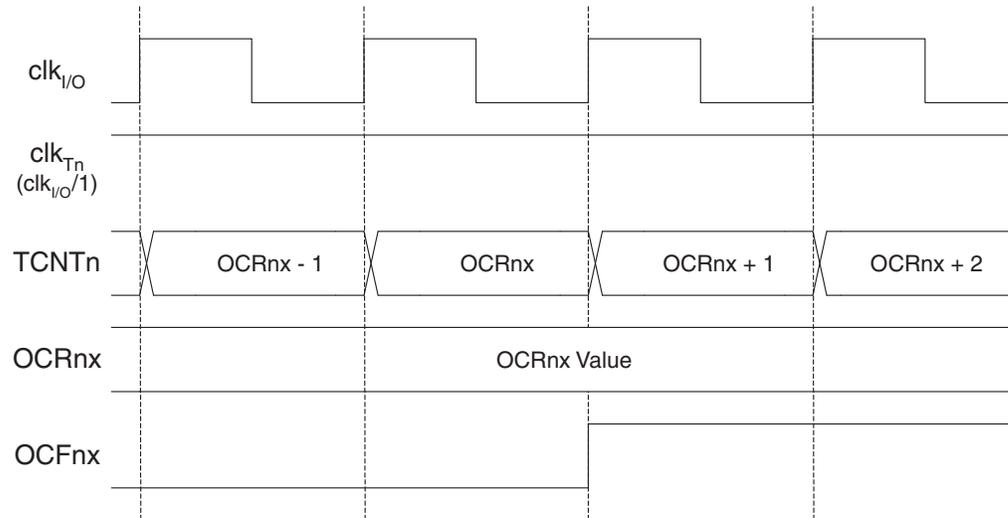
[Figure 50](#) shows the same timing data, but with the prescaler enabled.
