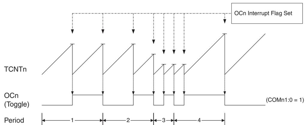
An interrupt can be generated each time the counter value reaches the TOP value by using the OCF0 Flag. If the interrupt is enabled, the interrupt handler routine can be used for updating the TOP value. However, changing TOP to a value close to BOTTOM when the counter is running with none or a low prescaler value must be done with care since the CTC mode does not have
