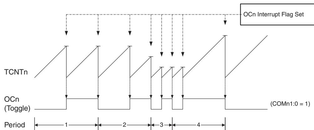
An interrupt can be generated each time the counter value reaches the TOP value by using the OCF2 Flag. If the interrupt is enabled, the interrupt handler routine can be used for updating the TOP value. However, changing the TOP to a value close to BOTTOM when the counter is running with none or a low prescaler value must be done with care since the CTC mode does not have the double buffering feature. If the new value written to OCR2 is lower than the current
