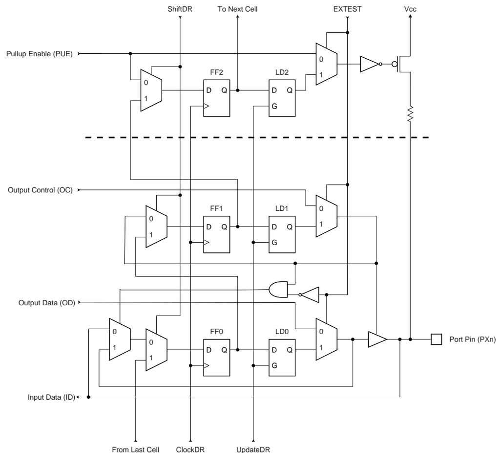
**Figure 117. General Port Pin Schematic Diagram<sup>(1)</sup>**
