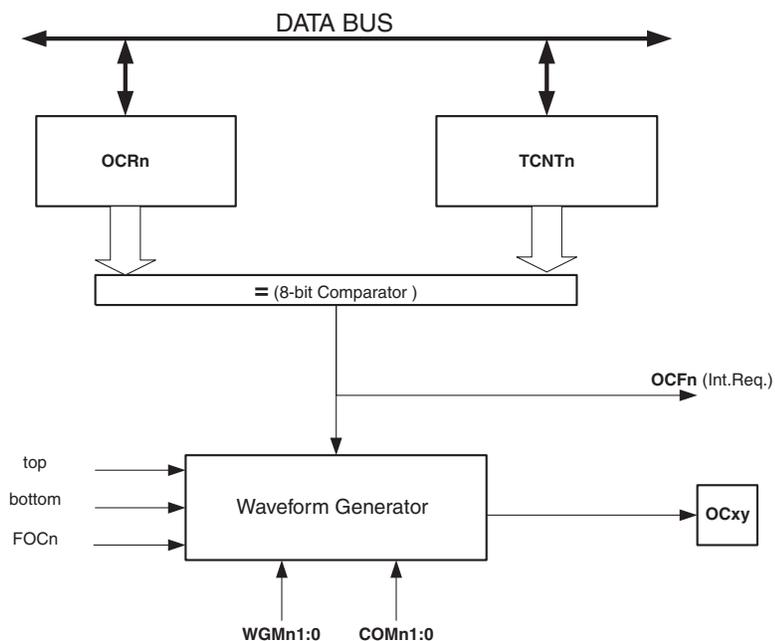
The OCR2 Register is double buffered when using any of the Pulse Width Modulation (PWM) modes. For the normal and Clear Timer on Compare (CTC) modes of operation, the double buffering is disabled. The double buffering synchronizes the update of the OCR2 Compare Register
