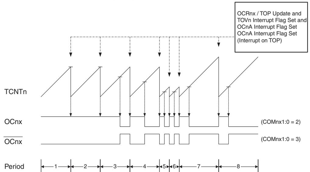
The Timer/Counter Overflow Flag (TOV1) is set each time the counter reaches TOP. In addition the OC1A or ICF1 Flag is set at the same timer clock cycle as TOV1 is set when either OCR1A or ICR1 is used for defining the TOP value. If one of the interrupts are enabled, the interrupt handler routine can be used for updating the TOP and compare values.
