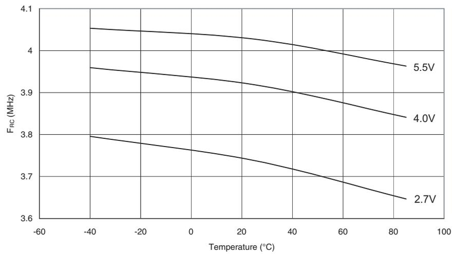
**Figure 198.** Calibrated 4 MHz RC Oscillator Frequency vs.  $V_{CC}$
