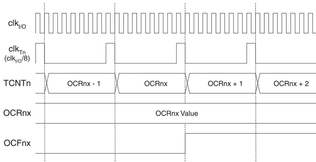
[Figure 51](#) shows the count sequence close to TOP in various modes. When using phase and frequency correct PWM mode the OCR1x Register is updated at BOTTOM. The timing diagrams
