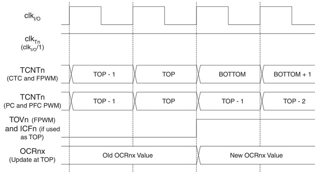
Figure 52 shows the same timing data, but with the prescaler enabled.
