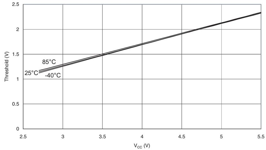
**Figure 187.** Reset Input Pin Hysteresis vs.  $V_{CC}$
