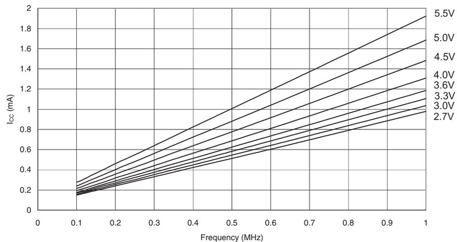
**Figure 150.** Active Supply Current vs. Frequency (1 MHz - 20 MHz)
