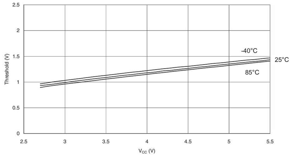
**Figure 184.** I/O Pin Input Hysteresis vs.  $V_{CC}$
