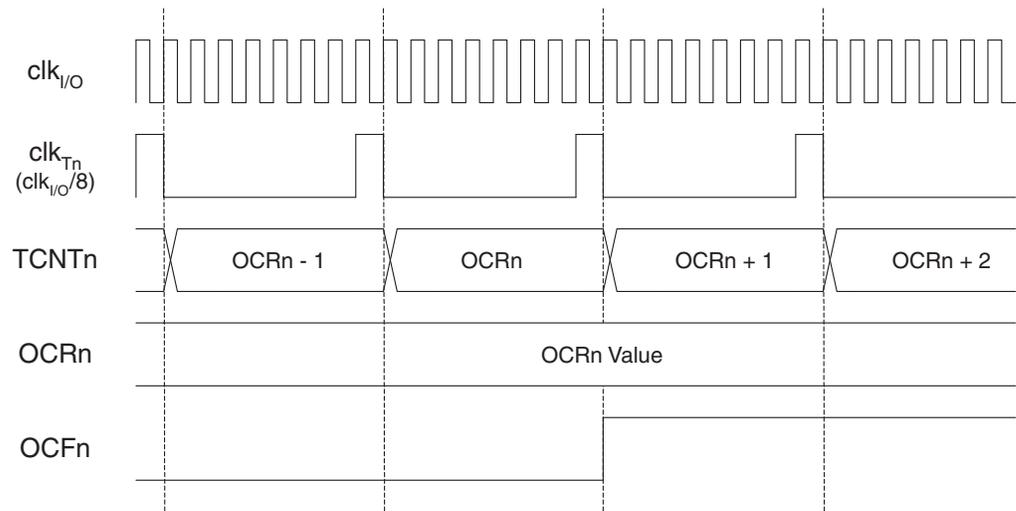
Figure 63 shows the setting of OCF2 and the clearing of TCNT2 in CTC mode.
