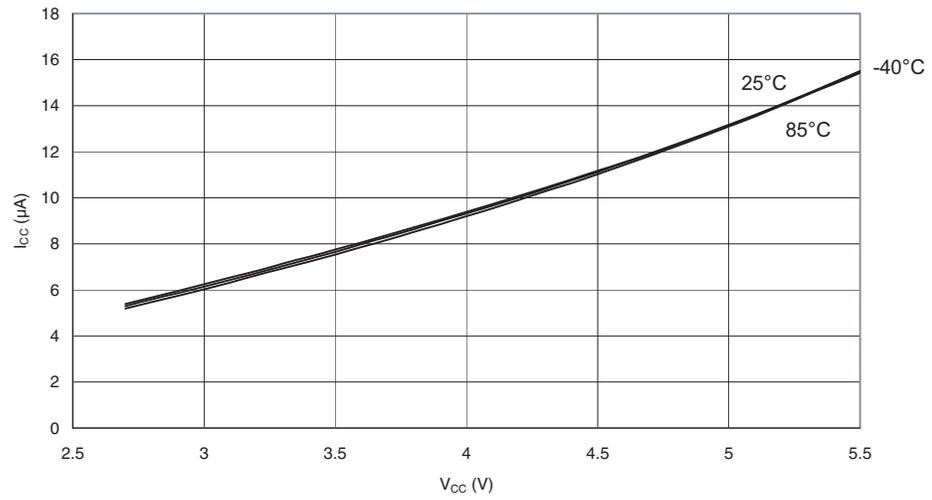
**Figure 211.** Programming Current vs.  $V_{CC}$
