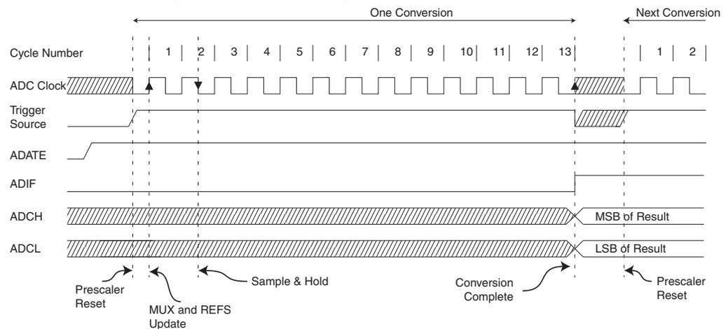
**Figure 104. ADC Timing Diagram, Free Running Conversion**
