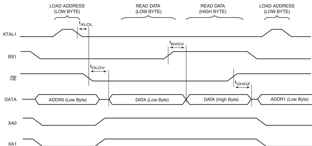
Note: 1. The timing requirements shown in Figure 133 (that is,  $t_{DVXH}$ ,  $t_{XHXL}$ , and  $t_{XLDX}$ ) also apply to reading operation.
