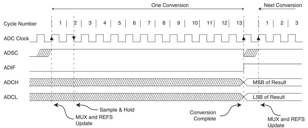
**Figure 103. ADC Timing Diagram, Auto Triggered Conversion**
