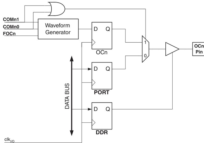
The general I/O port function is overridden by the Output Compare (OC0) from the Waveform Generator if either of the COM01:0 bits are set. However, the OC0 pin direction (input or output) is still controlled by the Data Direction Register (DDR) for the port pin. The Data Direction Register bit for the OC0 pin (DDR\_OC0) must be set as output before the OC0 value is visible on the pin. The port override function is independent of the Waveform Generation mode.
