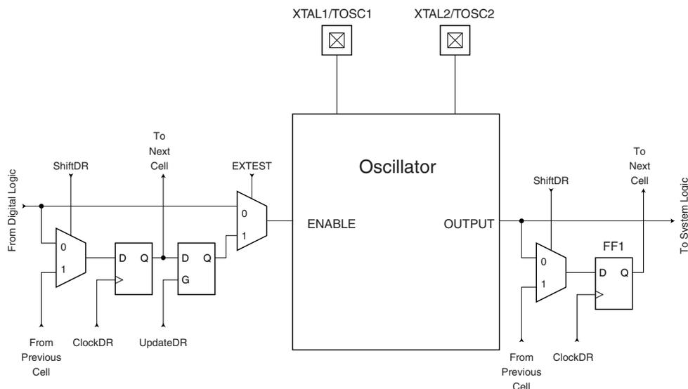
Table 90 summarizes the scan registers for the external clock pin XTAL1, Oscillators with XTAL1/XTAL2 connections as well as 32 kHz Timer Oscillator.
