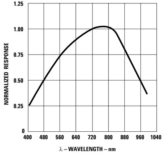
Figure 18. Receiver Spectral Response Normalized to 820 nm.
