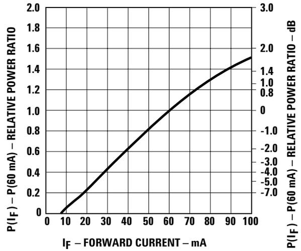
Figure 10. Normalized Transmitter Output vs. Forward Current.
