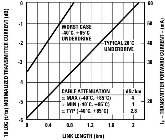
Figure 5. HFBR-14x4Z/HFBR-24x2Z Link Design Limits with 50/125  $\mu$ m Cable.
