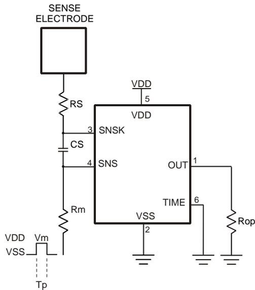
**Figure 3.8 Override Pulse (Delay Multiplier x24)**
