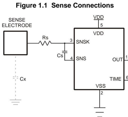
For optimum noise immunity, the electrode should only be connected to the SNSK pin.
