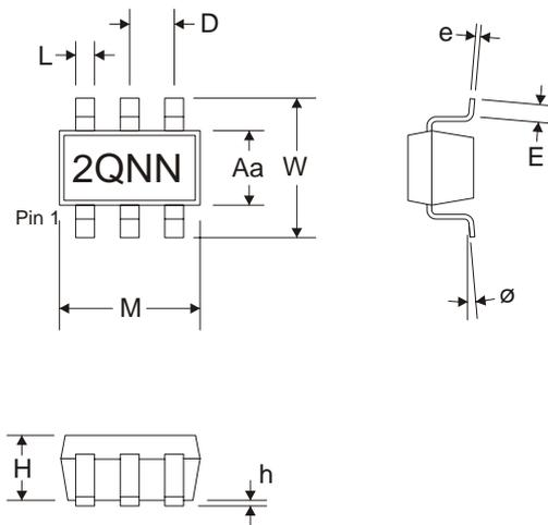
**Note:** the part marking shown is for high volume parts. Samples may be shipped marked 02NN.
