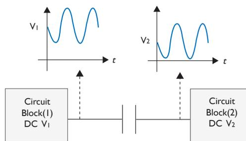
Coupling capacitor separates DC voltages of circuit blocks but couples AC signal.
