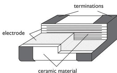
Surface mount multilayer ceramic capacitor construction
