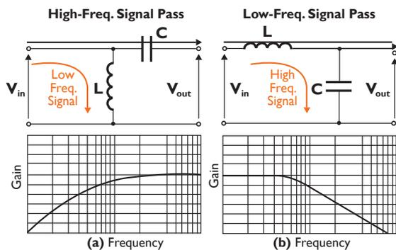
Filtering functions of capacitor coupled with inductor
