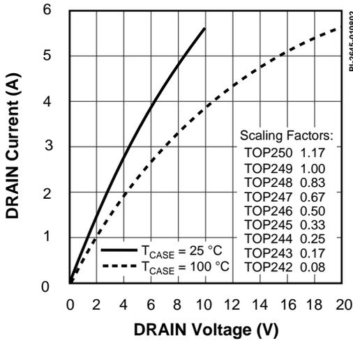
Figure 66. Output Characteristics.
