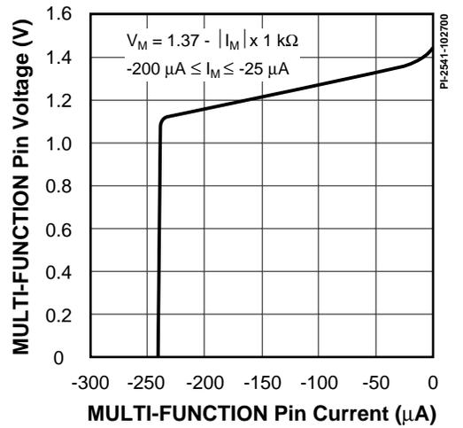
Figure 63b. MULTI-FUNCTION Pin Voltage vs. Current (Expanded).
