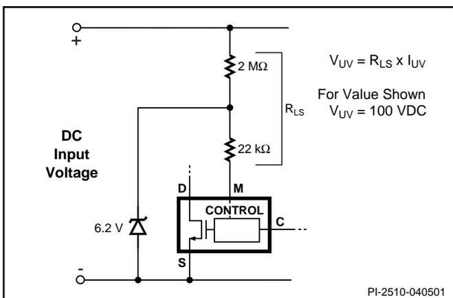
Figure 32. Line Sensing for Under-Voltage Only (Overvoltage Disabled).
