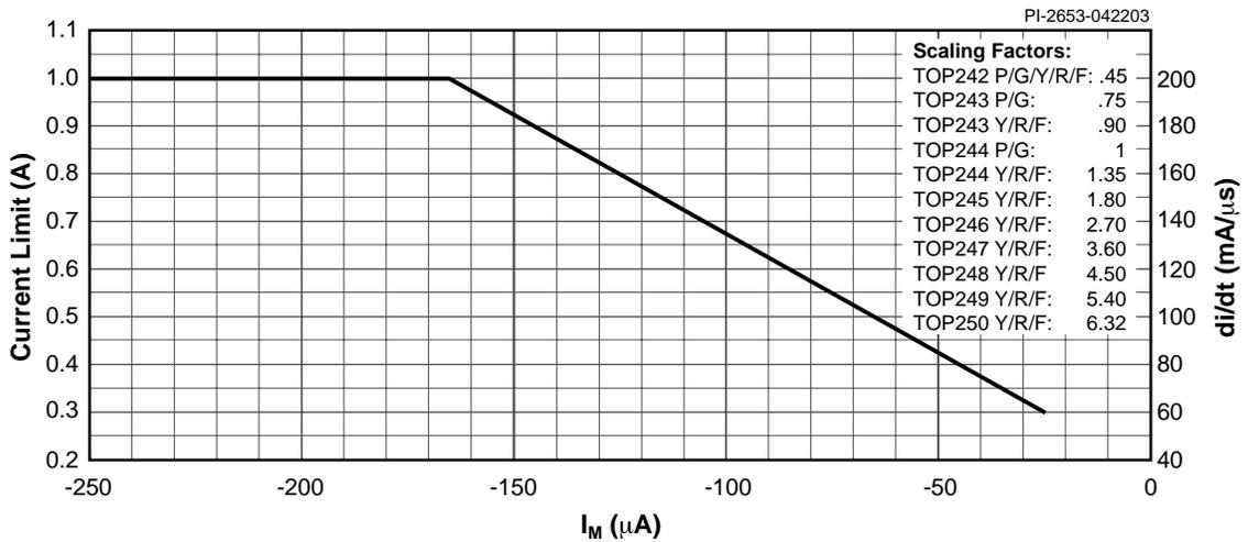
Figure 54. Current Limit vs. MULTI-FUNCTION Pin Current.
