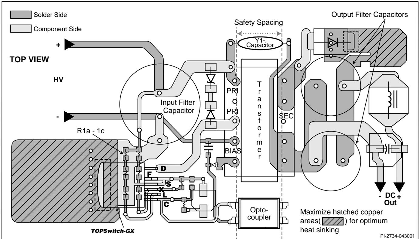
Figure 49. Layout Considerations for TOPSwitch-GX using R Package.
