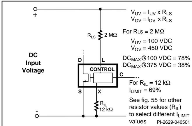
Figure 28. Line-Sensing and Externally Set Current Limit.
