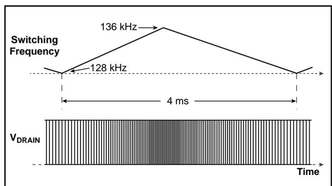
Figure 9. Switching Frequency Jitter (Idealized  $V_{DRAIN}$  waveform).
