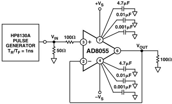
TPC 1. Test Circuit,  $G = +1$ ,  $R_L = 100 \Omega$
