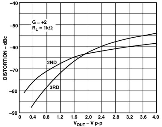
TPC 12. Distortion vs.  $V_{OUT}$  @ 20 MHz
