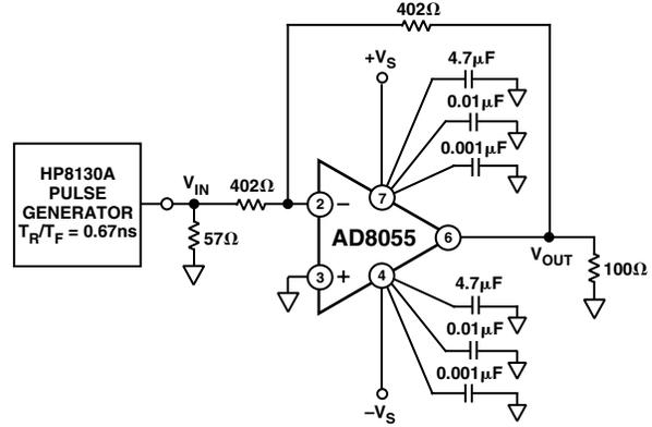
TPC 4. Test Circuit,  $G = -1$ ,  $R_L = 100 \Omega$
