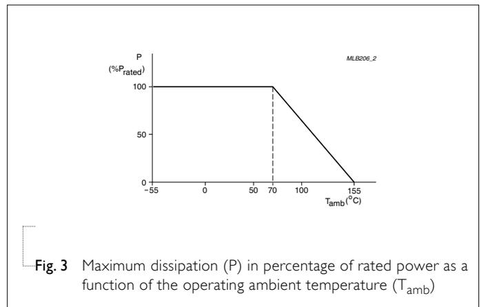
Fig. 3 Maximum dissipation (P) in percentage of rated power as a function of the operating ambient temperature (T<sub>amb</sub>)
