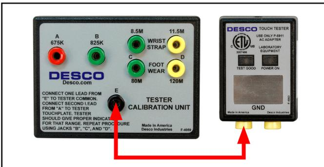
Figure 8. Connecting the test lead from banana jack “E” on the Calibration Unit to one of the banana jacks on the Wrist Strap Touch Tester
