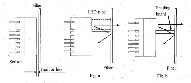
Acrylic or Polycarbonate resin would be recommended as the material of the filter. Please be careful to use ABS resin or molded transparent resin with coating since there is a possibility to be a cause of operating error by reflected light reaches to the detector inside of the filter.
