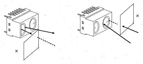
2) Detectable area characteristics of GP2Y0D810Z0F as example is following.
