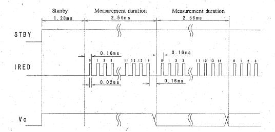
LED in these sensor emits maximum 15 times (4 times data sampling per one emission) and the sensor stop the LED emission once the output is settled by having 30 times detection or non-detection. So the minimum LED emission is 8 times for the shortest operation and the maximum LED emission is 15 times for the longest operation.
