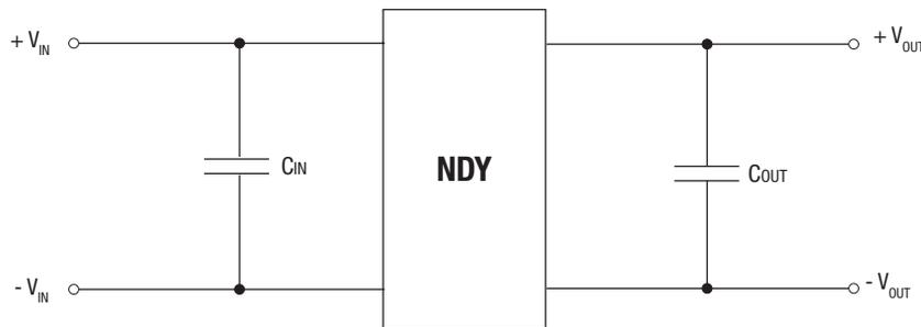
Recommended circuit for reduced ripple 3.3V output
