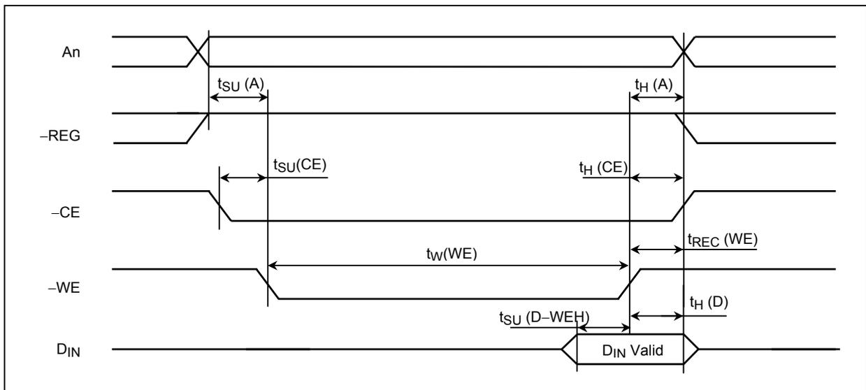
True IDE Mode IO Read/Write AC Characteristics
