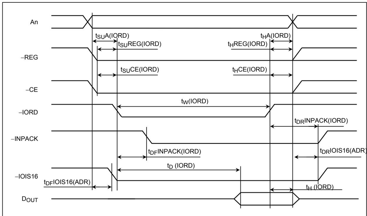
I/O Access Write AC Characteristics
