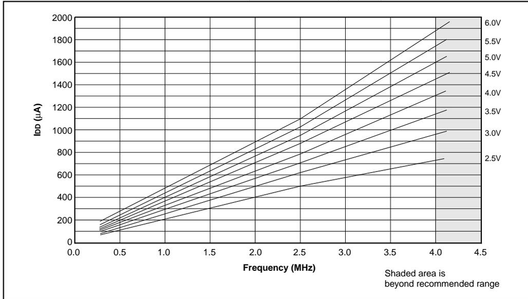
**FIGURE 14-13: MAXIMUM I<sub>DD</sub> vs. FREQUENCY (RC MODE @ 22 pF, -40°C TO 85°C)**
