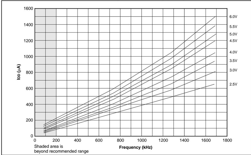
FIGURE 14-15: MAXIMUM I<sub>DD</sub> vs. FREQUENCY (RC MODE @ 100 pF, -40°C TO 85°C)
