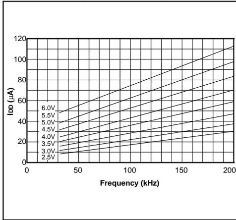
**FIGURE 14-27: TYPICAL  $I_{DD}$  vs. FREQUENCY
