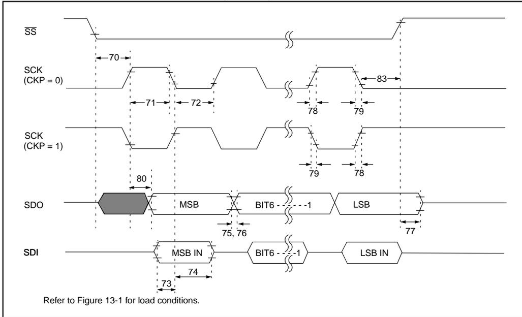
**FIGURE 13-11: SPI SLAVE MODE TIMING (CKE = 1)**
