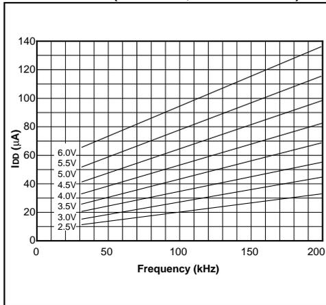
**FIGURE 14-28: MAXIMUM  $I_{DD}$  vs.
