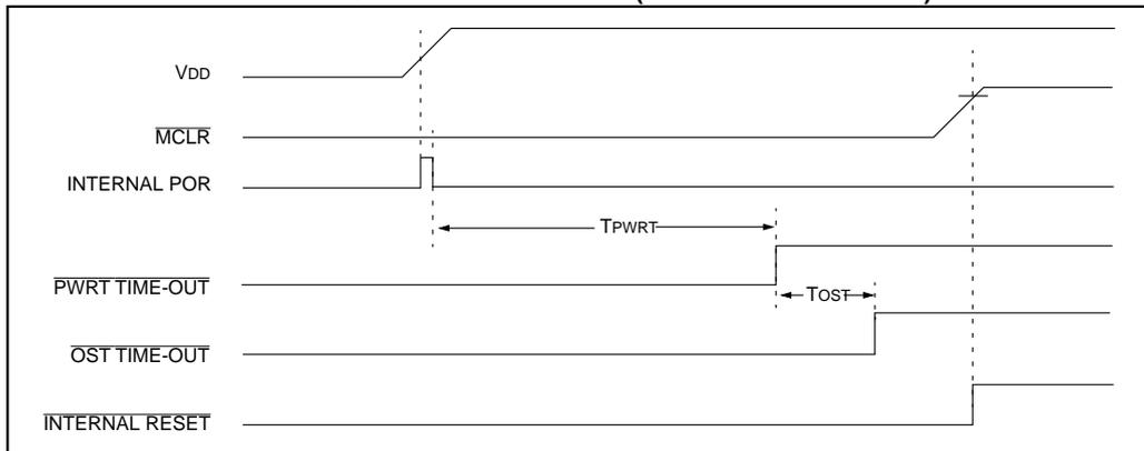
**FIGURE 10-10: SLOW RISE TIME ( $\overline{\text{MCLR}}$  TIED TO  $\text{V}_{\text{DD}}$ )**
