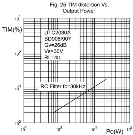
Fig. 25 TIM distortion Vs. Output Power
