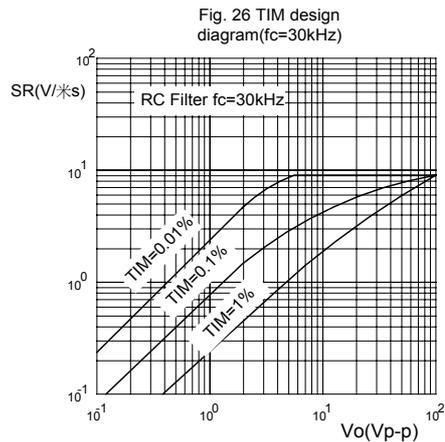
Fig. 26 TIM design diagram (fc=30kHz)
