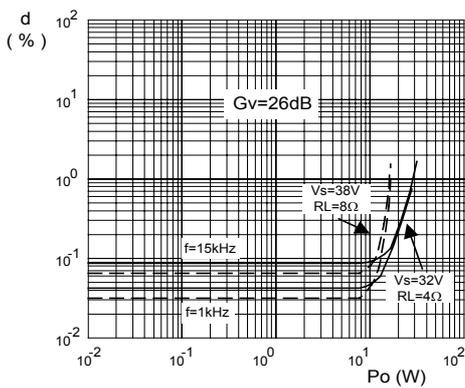
Fig.5 Two tone CCIF intermodulation distortion
