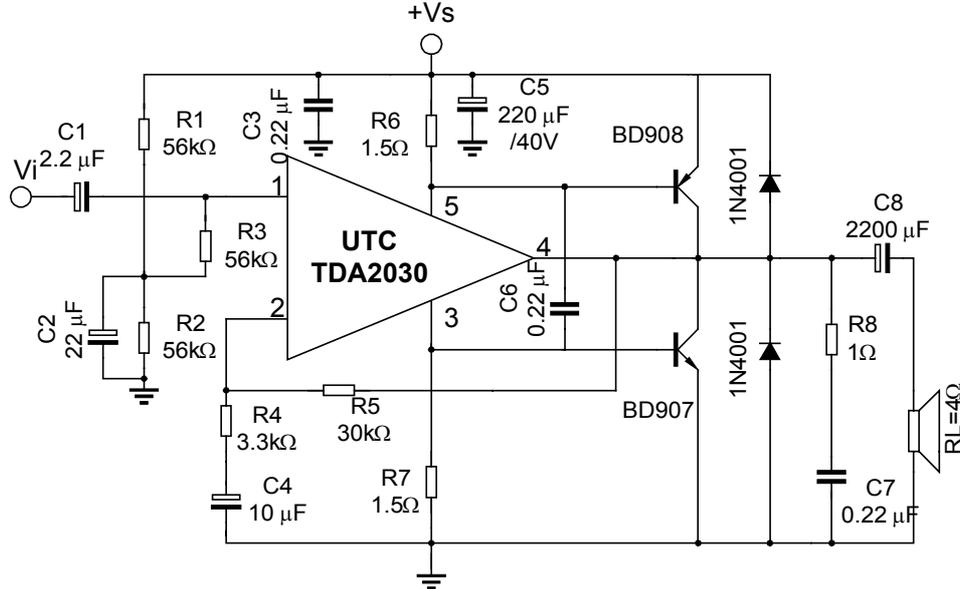
Fig. 8 Single supply high power amplifier(UTC TDA2030+BD908/BD907)
