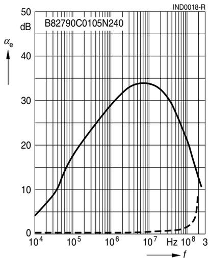
Insertion loss  $\alpha_e$  (typical values at  $Z = 50 \Omega$ )
