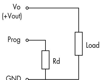
$$5 \text{ VDC input models: } Rd [\text{Ohm}] = \frac{21070}{Vo - 0.7525} - 5110$$
