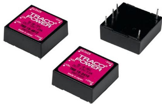
The THD-15 series is the latest generation of high performance 15W dc-dc converter modules setting new standards concerning power density. This product comes in a encapsulated package with dimensions of only 25.4 x 25.4 x 10mm and therefore occupies 50%(!) less board space than existing 15W converters.
