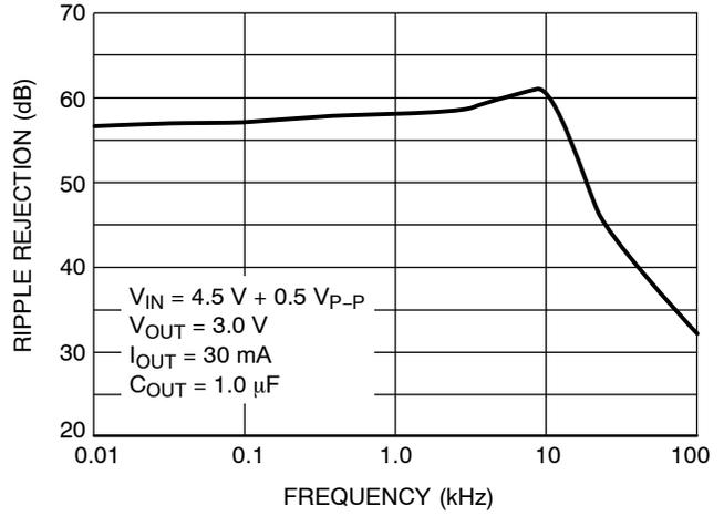
Figure 7. Ripple Rejection/Frequency
