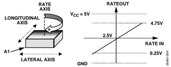
Figure 5. RATEOUT Signal Increases with Clockwise Rotation
