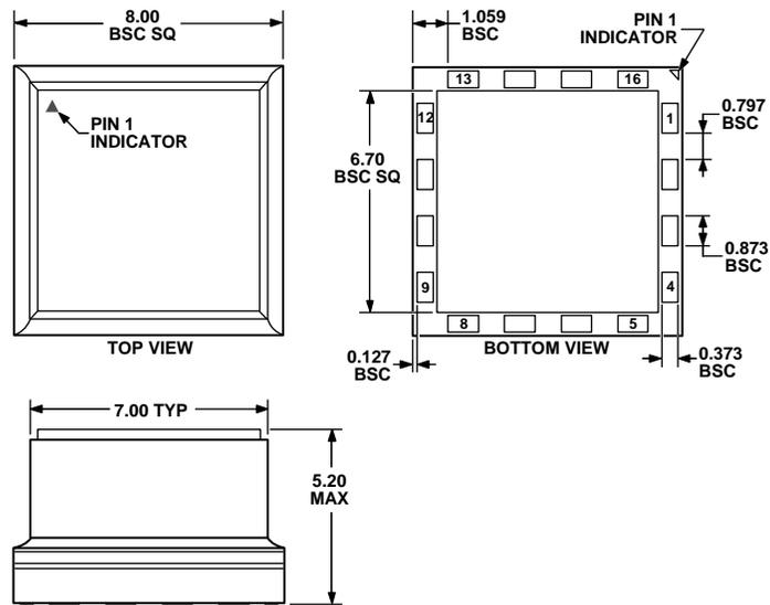
Figure 6. 16-Terminal Land Grid Array [LGA]
