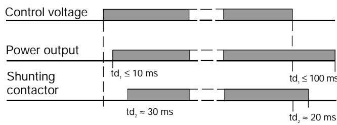
$t_{D1}$  = time delay semiconductor
