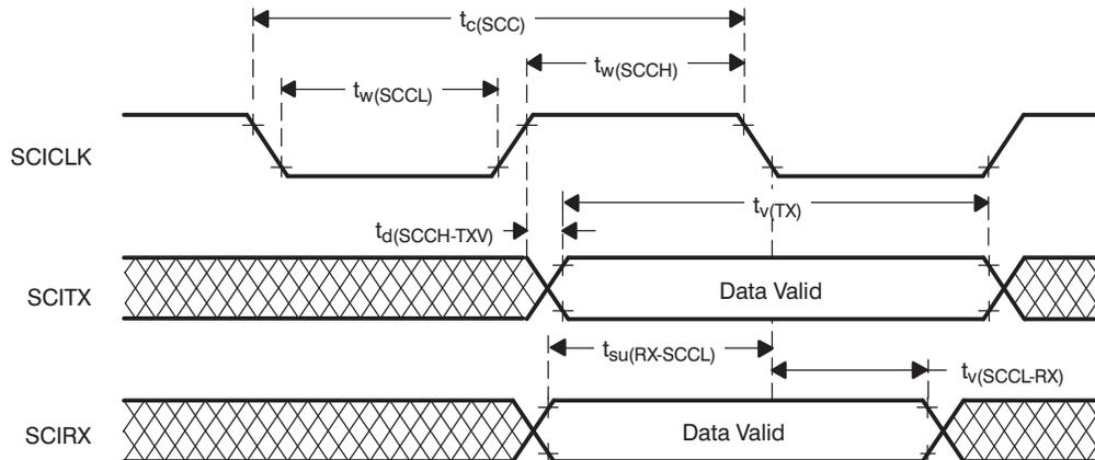
A. Data transmission/reception characteristics for isosynchronous mode with internal clocking are similar to the asynchronous mode. Data transmission occurs on the SCI<sub>n</sub>CLK rising edge, and data reception occurs on the SCI<sub>n</sub>CLK falling edge.
