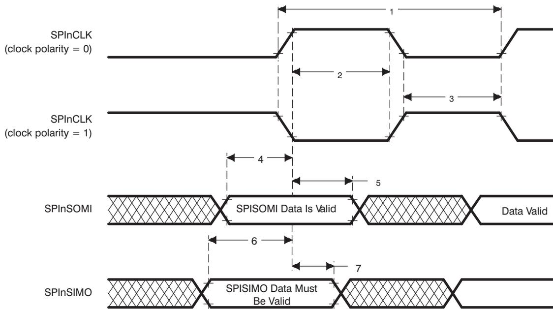
**Figure 15. SPIn Slave Mode External Timing (CLOCK PHASE = 1)**
