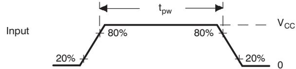
Figure 11. CMOS-Level Inputs
