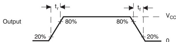
**Figure 10. CMOS-Level Outputs**
