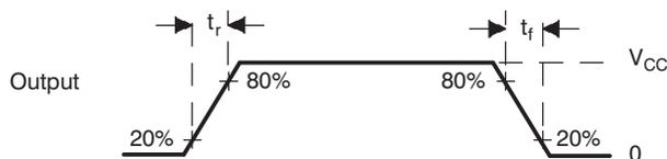
**Figure 10. CMOS-Level Outputs**
