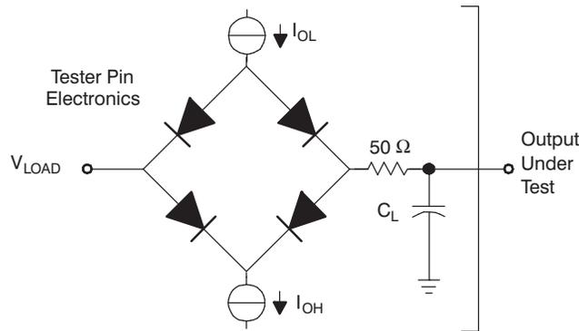
Where:  $I_{OL} = I_{OL\text{ MAX}}$  for the respective pin<sup>(A)</sup>
