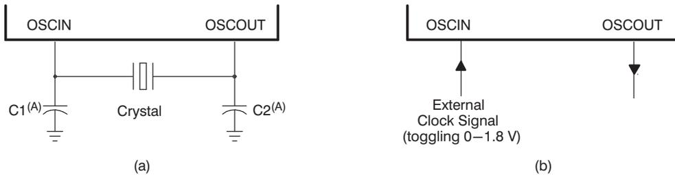
A. The values of C1 and C2 should be provided by the resonator/crystal vendor.
