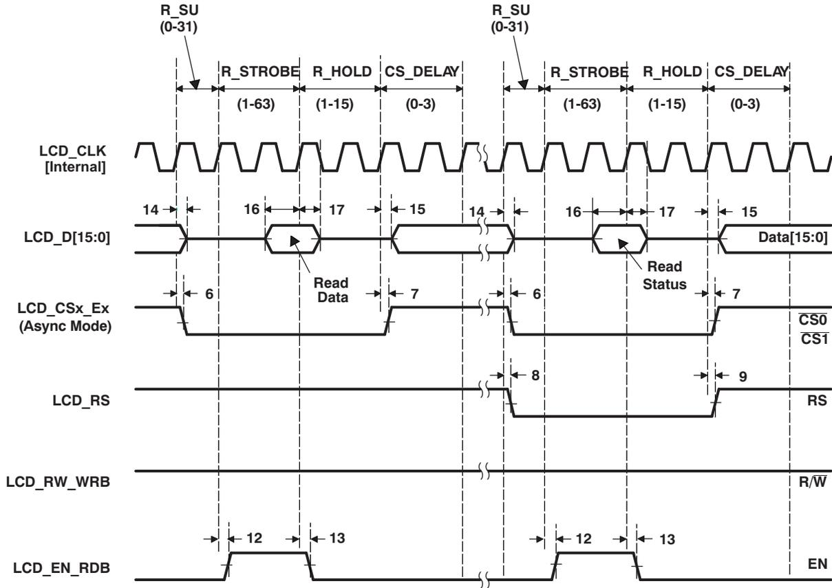
Figure 5-30. Micro-Interface Graphic Display 6800 Status
