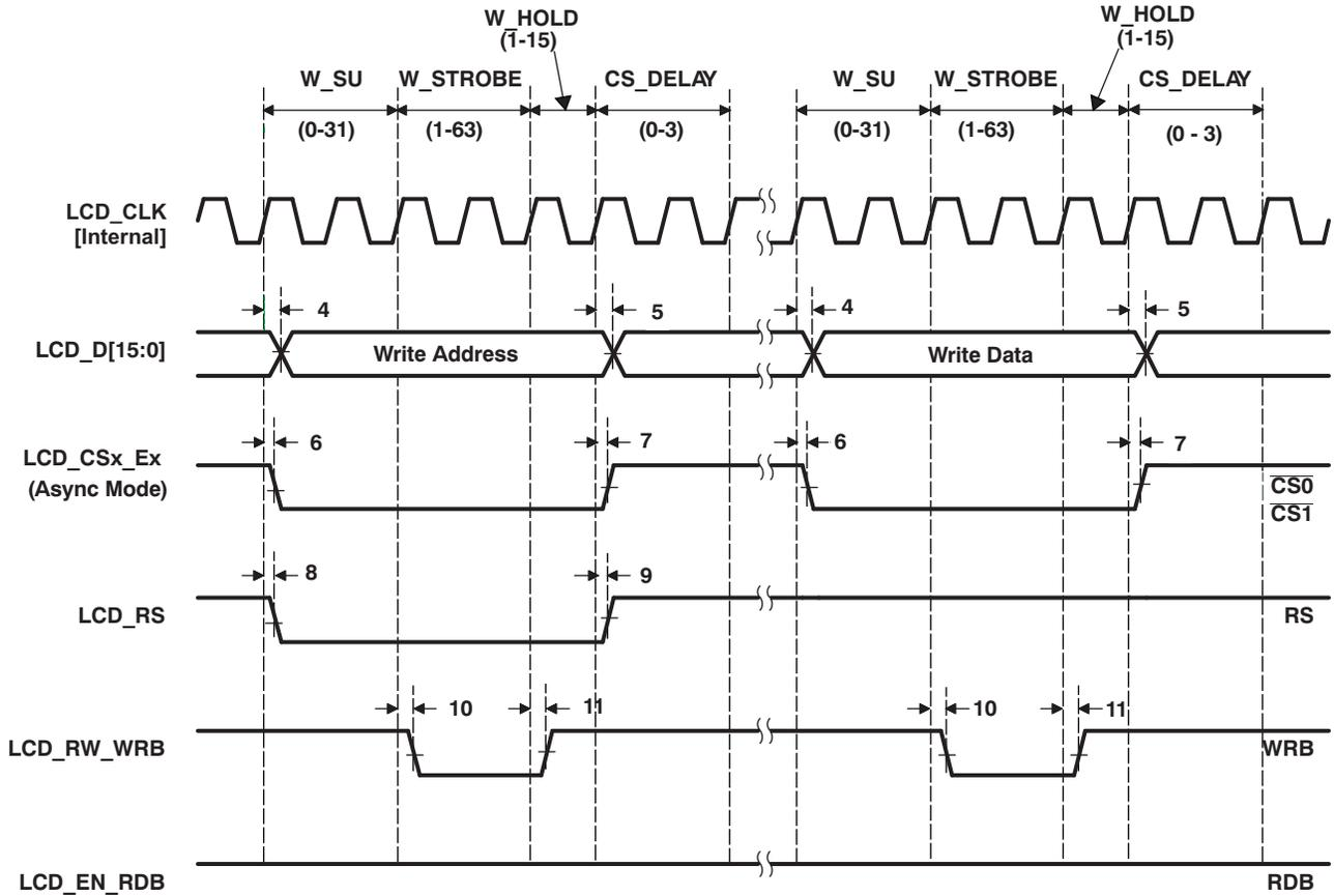
Figure 5-31. Micro-Interface Graphic Display 8080 Write
