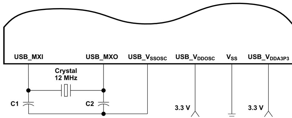
Figure 5-6. 12-MHz USB Oscillator
