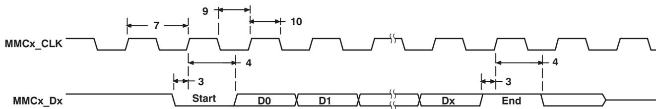
Figure 5-19. MMC/SD Card Response Timing
