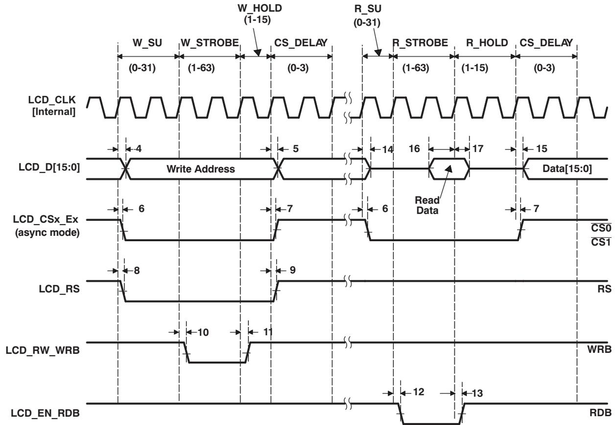
Figure 5-32. Micro-Interface Graphic Display 8080 Read
