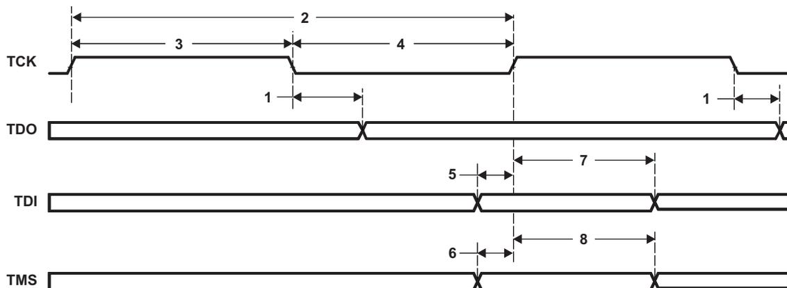
Figure 5-42. JTAG Test-Port Timing
