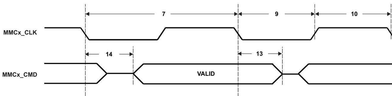
Figure 5-18. MMC/SD Host Command Write Timing
