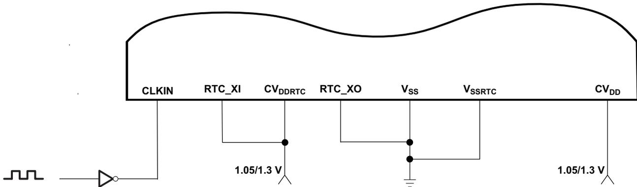
Figure 5-5. LVC MOS-Compatible Clock Input With RTC Oscillator Disabled
