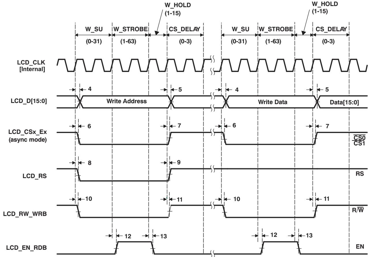
Figure 5-28. Micro-Interface Graphic Display 6800 Write
