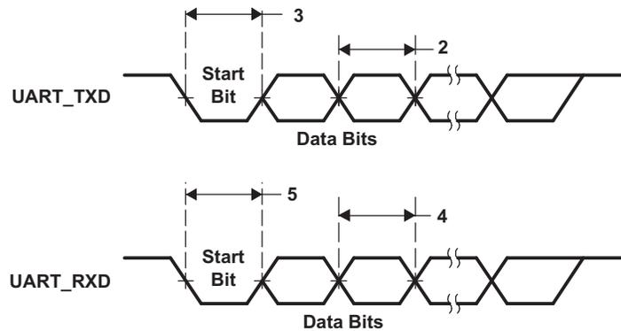
Figure 5-24. UART Transmit/Receive Timing
