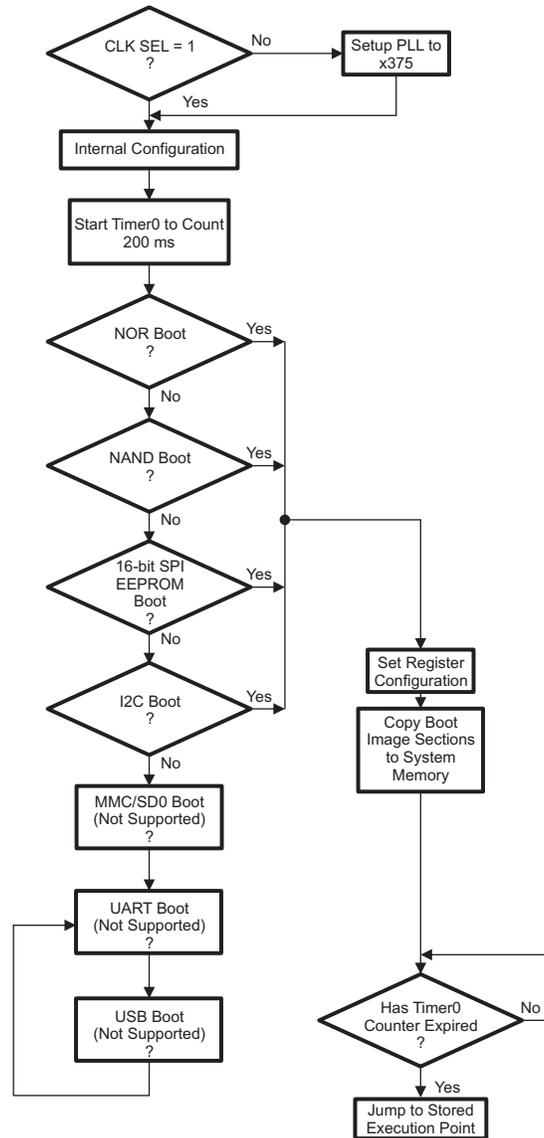
Figure 3-1. Bootloader Software Architecture
