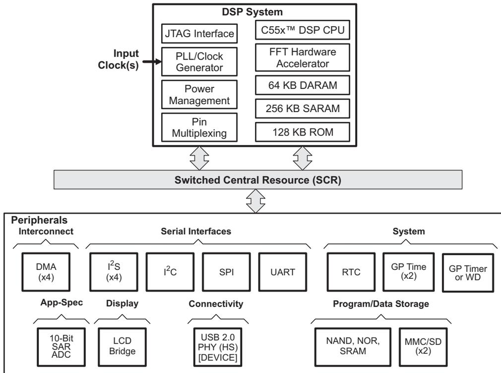
Figure 1-1. TMS320VC5505 Functional Block Diagram
