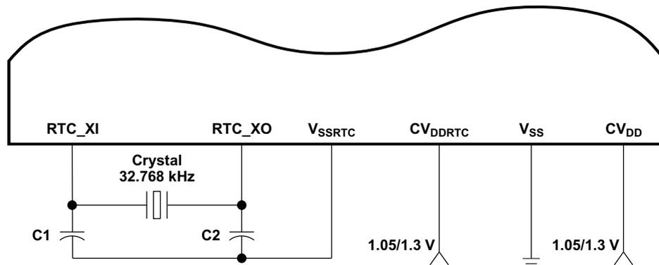
Figure 5-3. 32.768-kHz RTC Oscillator
