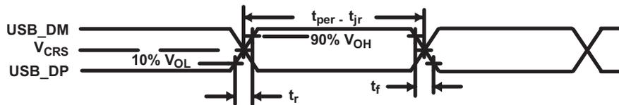
Figure 5-38. USB2.0 Integrated Transceiver Interface Timing
