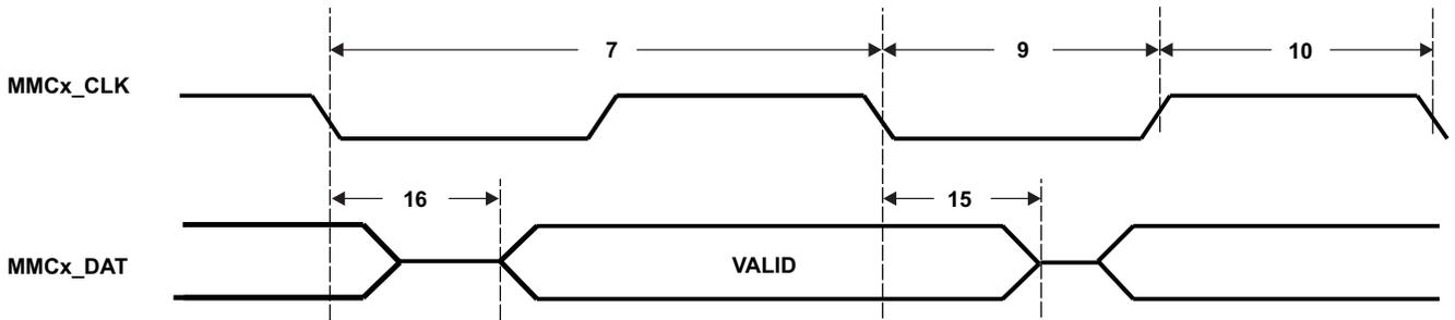
Figure 5-21. MMC/SD Data Write Timing
