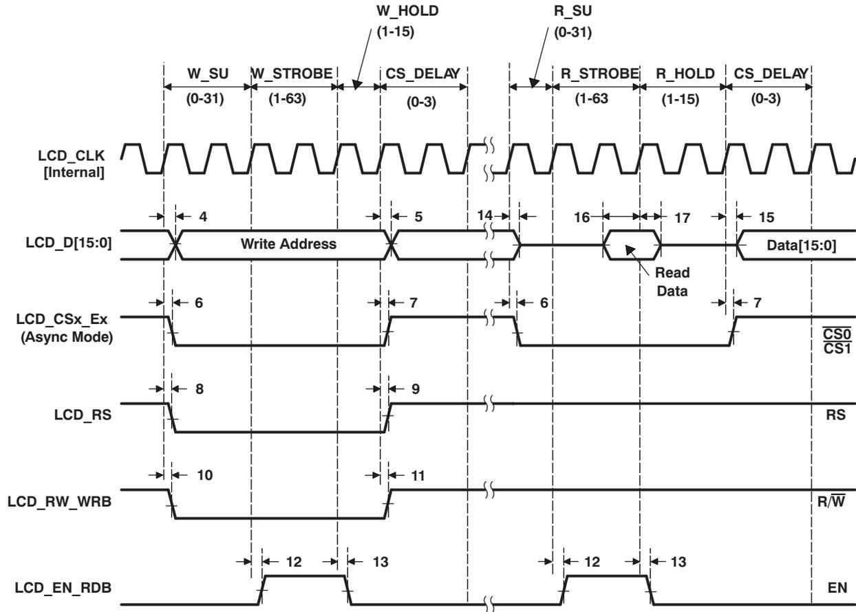
Figure 5-29. Micro-Interface Graphic Display 6800 Read
