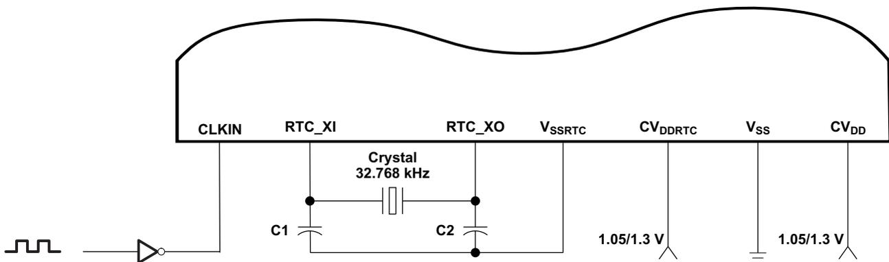
Figure 5-4. LVCMOS-Compatible Clock Input With RTC Oscillator Enabled
