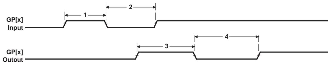
Figure 5-39. GPIO Port Timing
