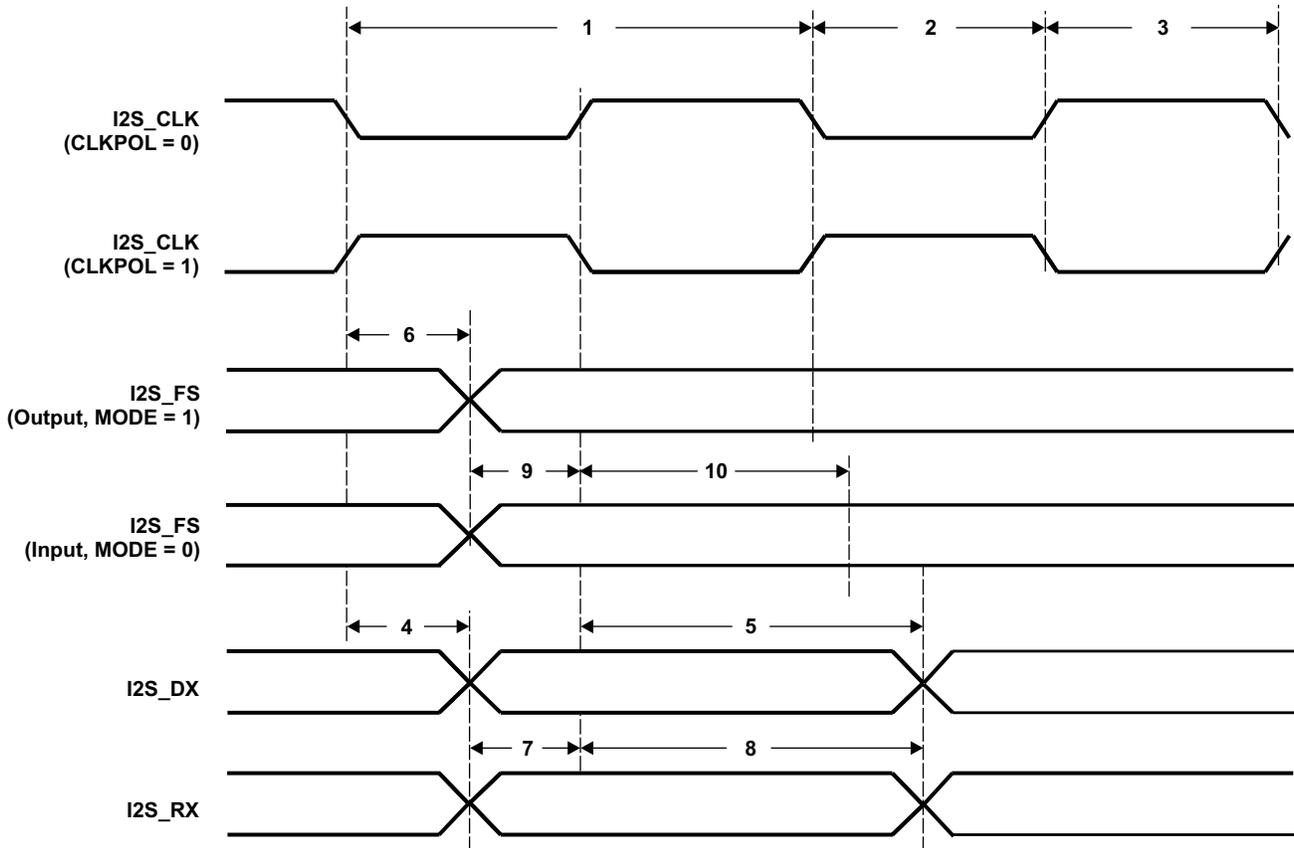
Figure 5-25. I2S Input and Output Timings
