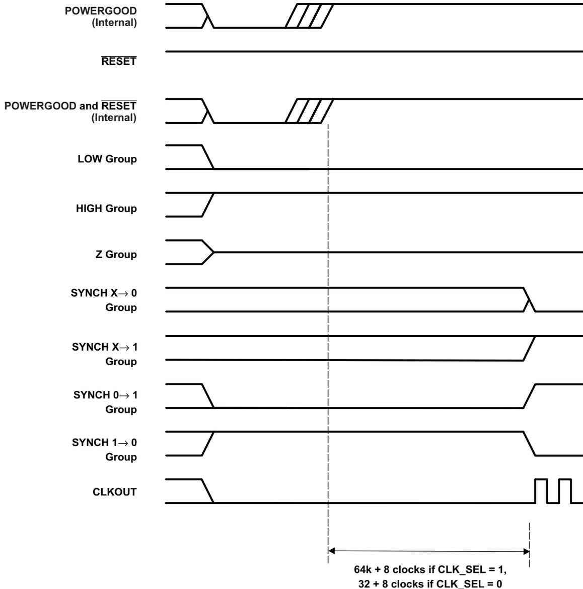
Figure 5-9. Power-On Reset Timing Requirements
