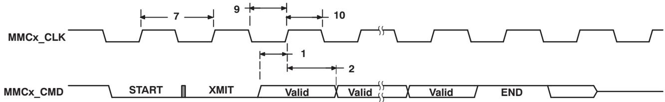
Figure 5-20. MMC/SD Host Write Timing
