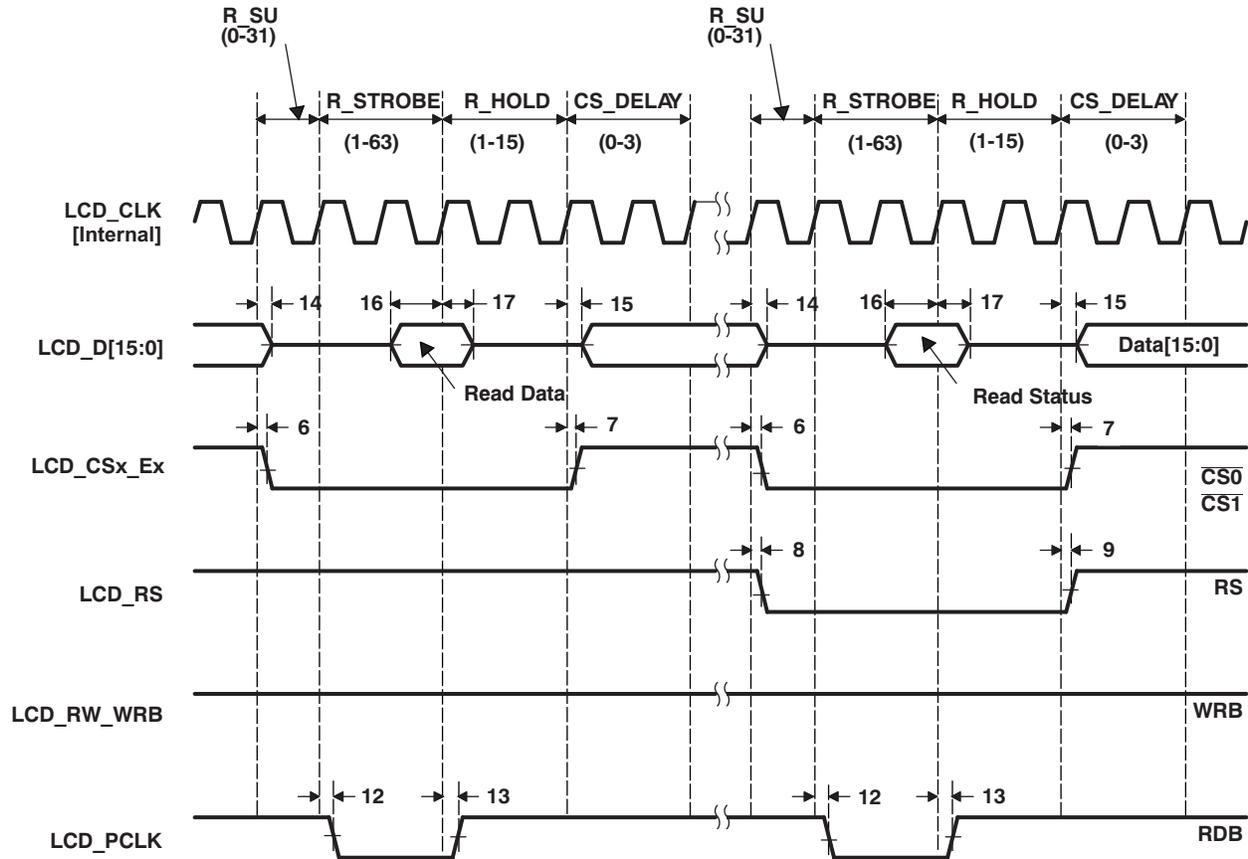
Figure 5-33. Micro-Interface Graphic Display 8080 Status
