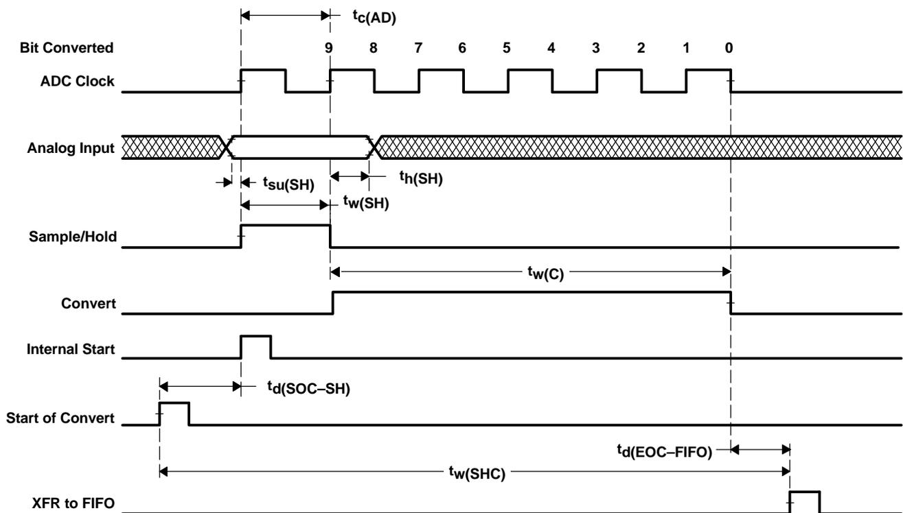
Figure 49. Analog-to-Digital Timing
