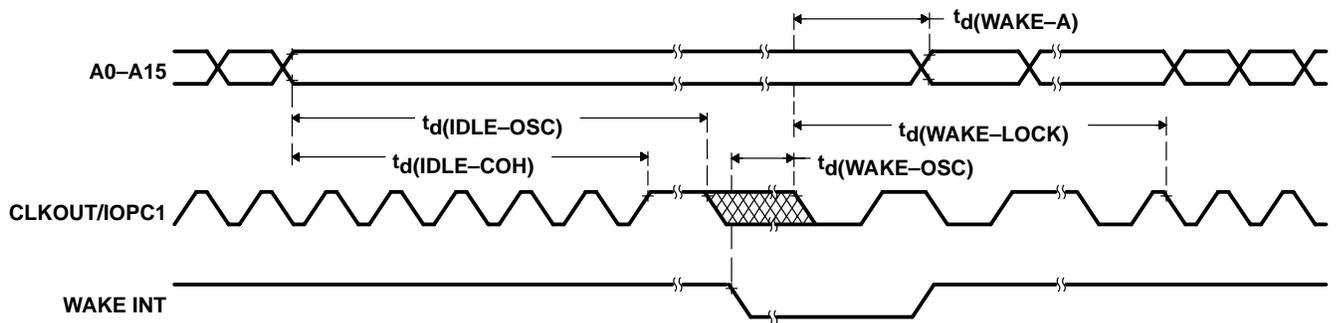
Figure 26. OSC Power-Down Entry and Exit Timings
