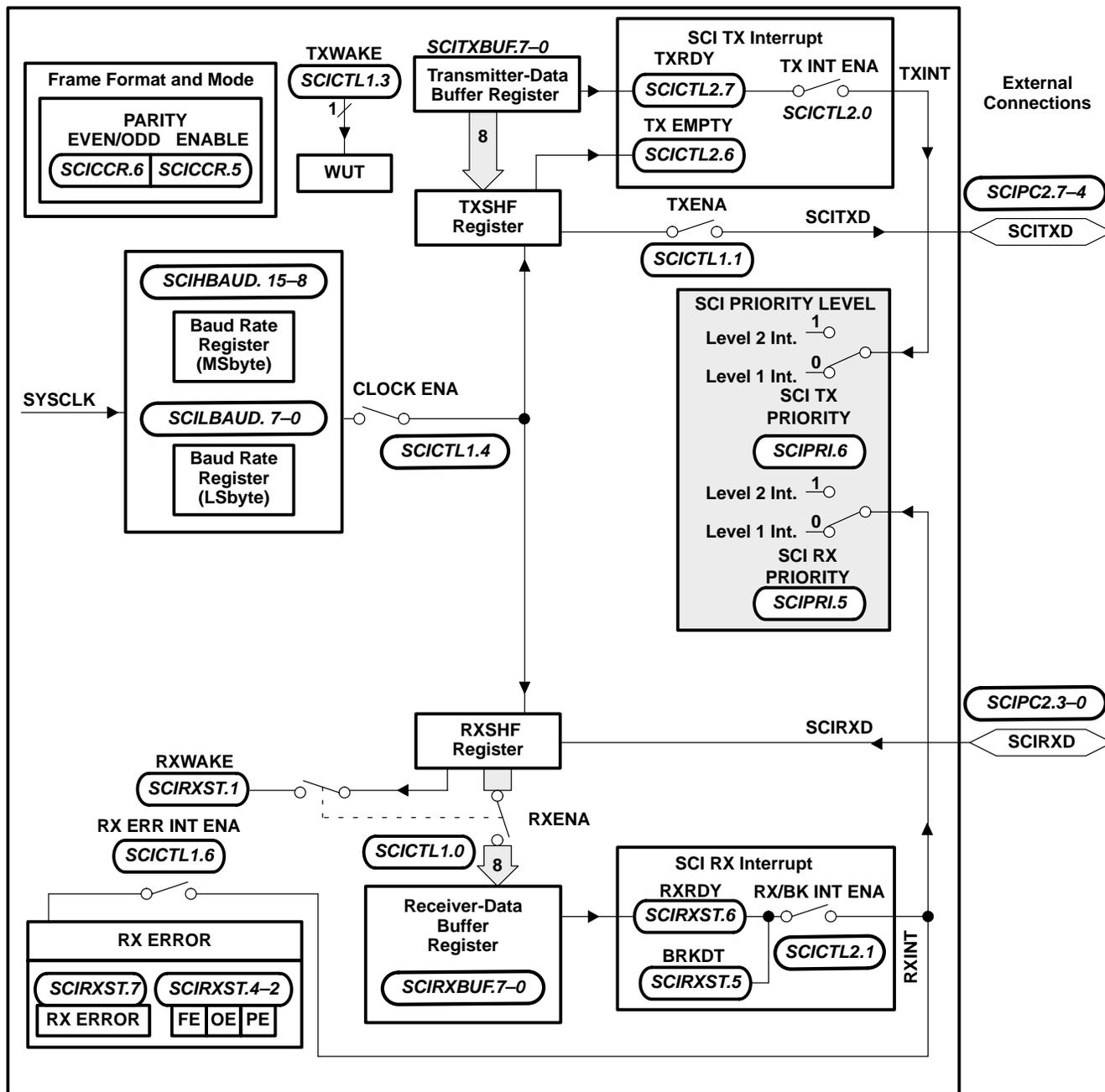
Figure 14. Serial Communications Interface (SCI) Module Block Diagram
