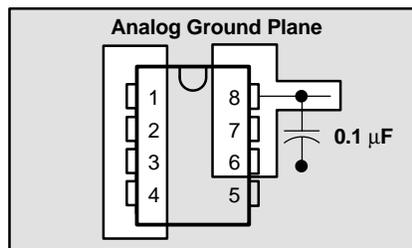
**Figure 16. Power-Supply Bypassing**
