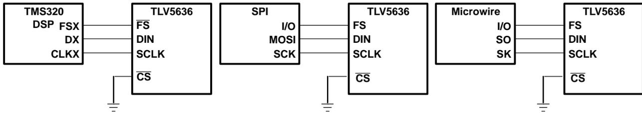
Figure 14. Three Wire Interface
