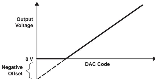
**Figure 19. Effect of Negative Offset (single supply)**
