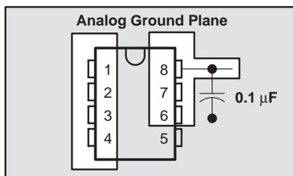
Figure 20. Power-Supply Bypassing
