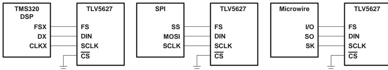
**Figure 16. Three-Wire Interface**
