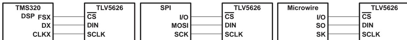
**Figure 13. Three-Wire Interface**
