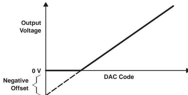
**Figure 14. Effect of Negative Offset (single supply)**
