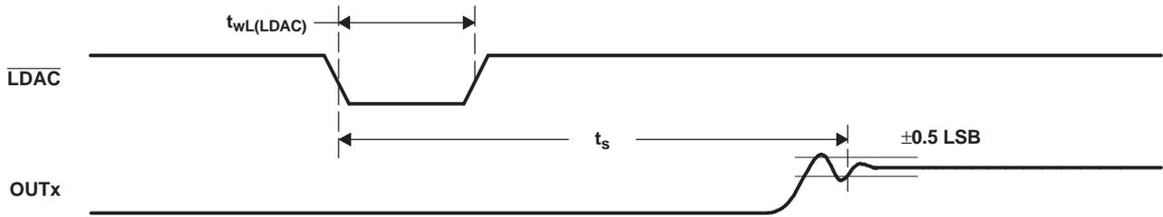
Figure 2. Output Timing
