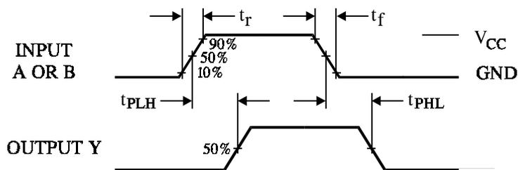
**Figure 1. Switching Waveforms**
