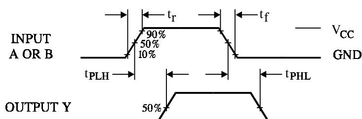
**Figure 1. Switching Waveforms**
