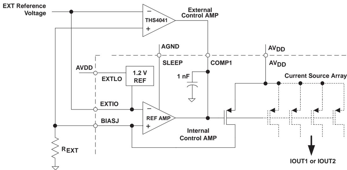
**Figure 31. Bypassing the Internal Reference and Control Amplifier**
