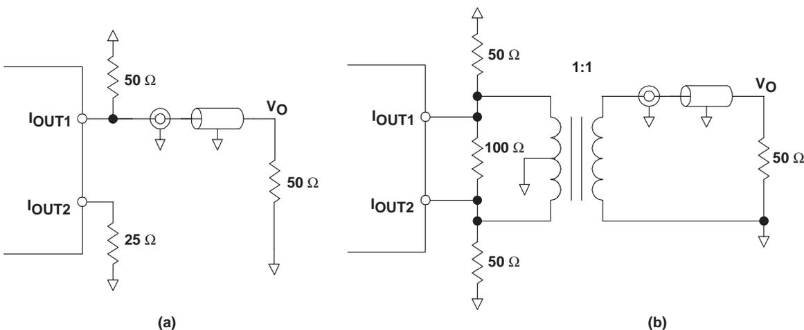
**Figure 34. Driving a Doubly Terminated 50 Ω Cable**
