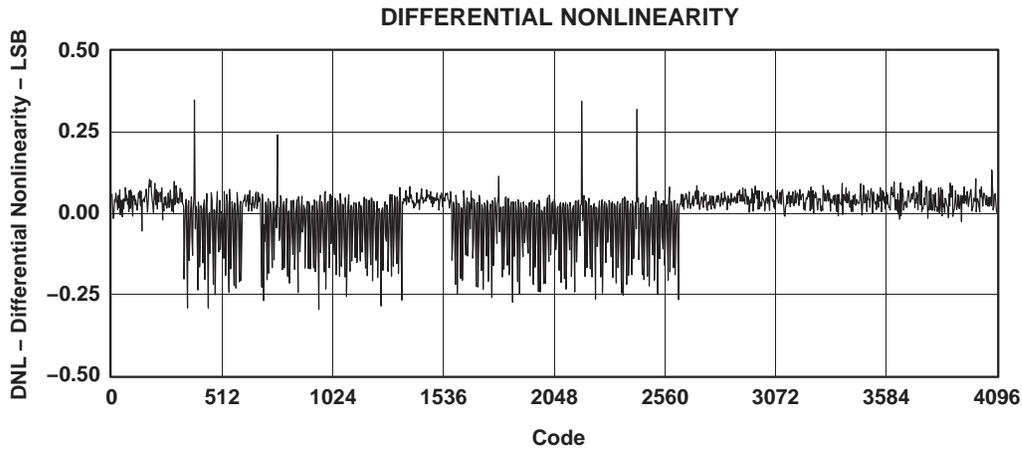
†  $V_{DD} = 5\text{ V}$ ,  $I_{OUTFS} = 20\text{ mA}$ , differential transformer coupled output,  $50\ \Omega$  doubly terminated load,  $T_A = 25^\circ\text{C}$  (unless otherwise noted.)
